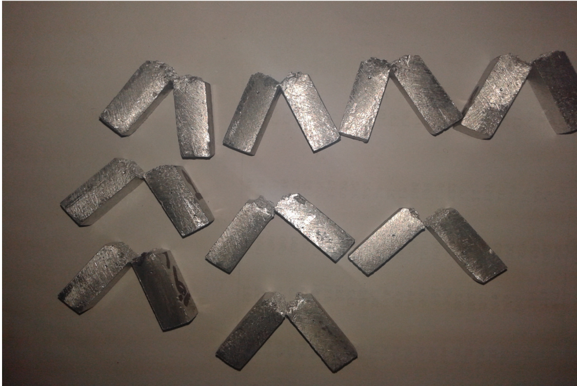
Figure 4.13: Broken piece of Impact test sample
