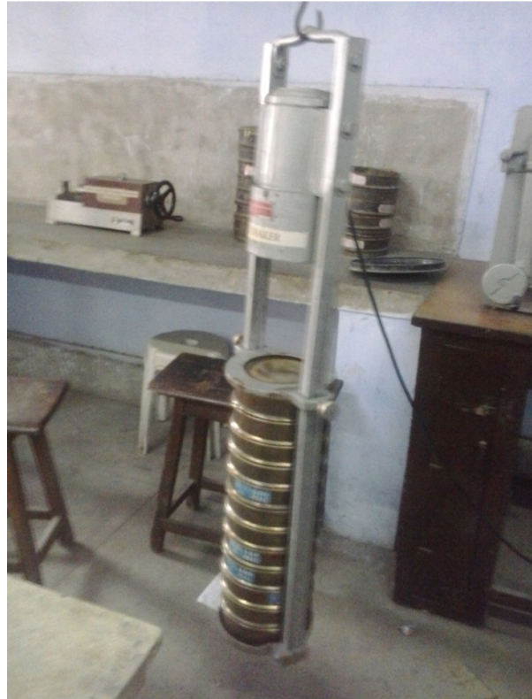
Figure 4.14: Sieve Shaker available at Sand Testing Lab at Thapar University.
