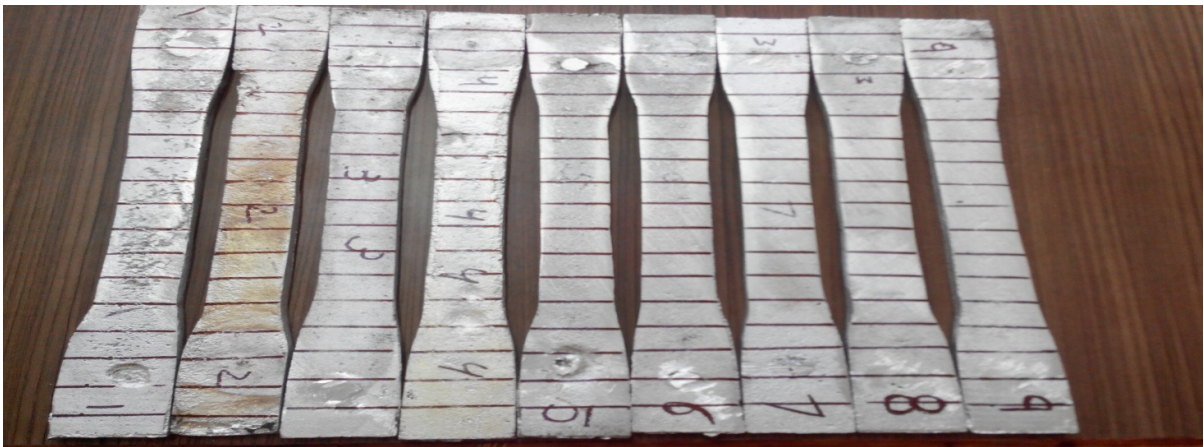
Figure 4.10: Samples made for Tensile Testing as per the ASTM E-8 standards
