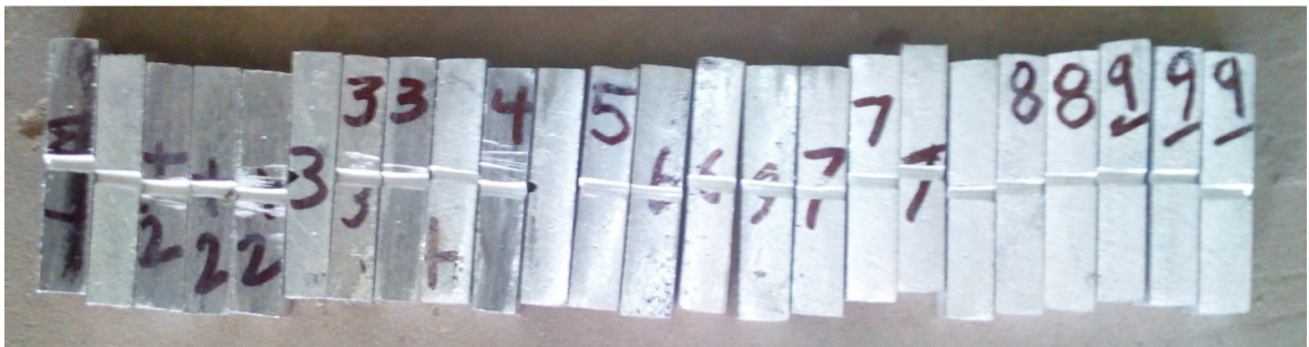
Figure 4.12: Samples made for impact test
