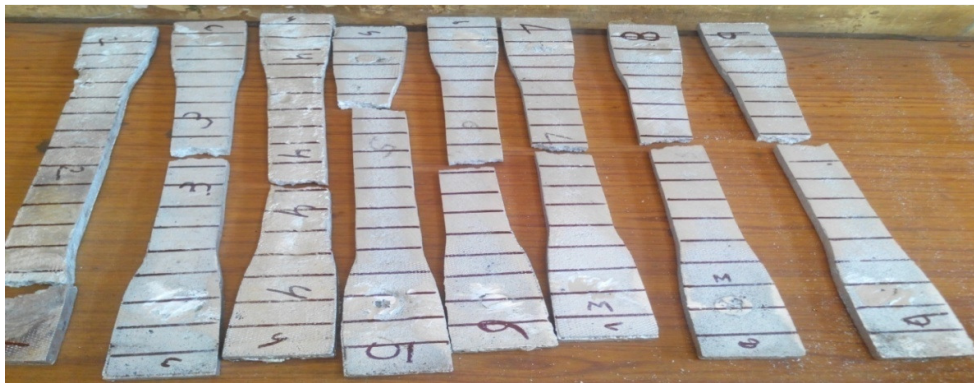
Figure 5.2: The broken samples of MMC using a computerized UTM testing machine as per the ASTM E-8 standards
