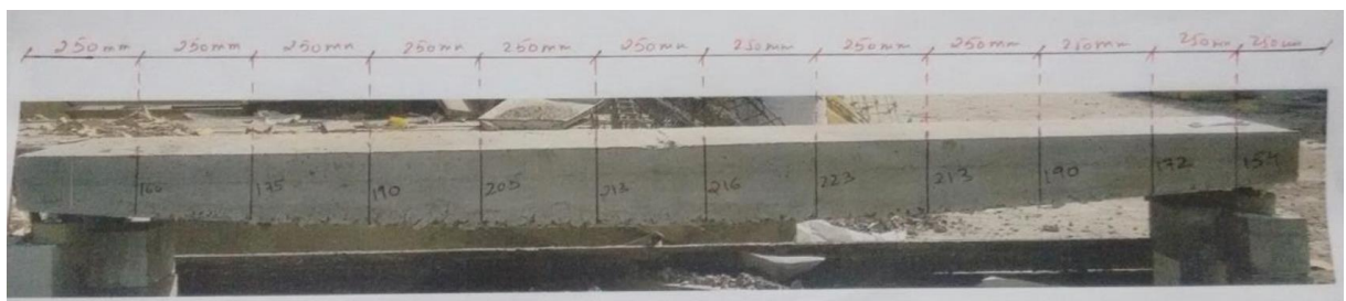
Fig.4.4 Deflection at Different Points for CG
