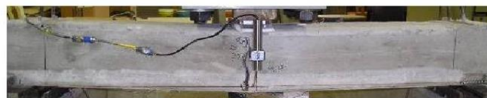
d) Flexural failure of specimen C1
