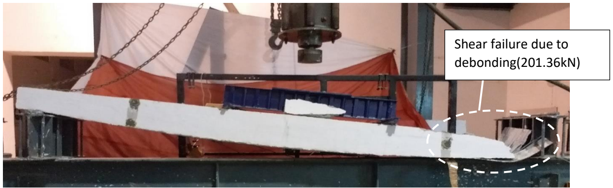
Fig.4.20 Failure Mode of CA Slab at 201.36kN
