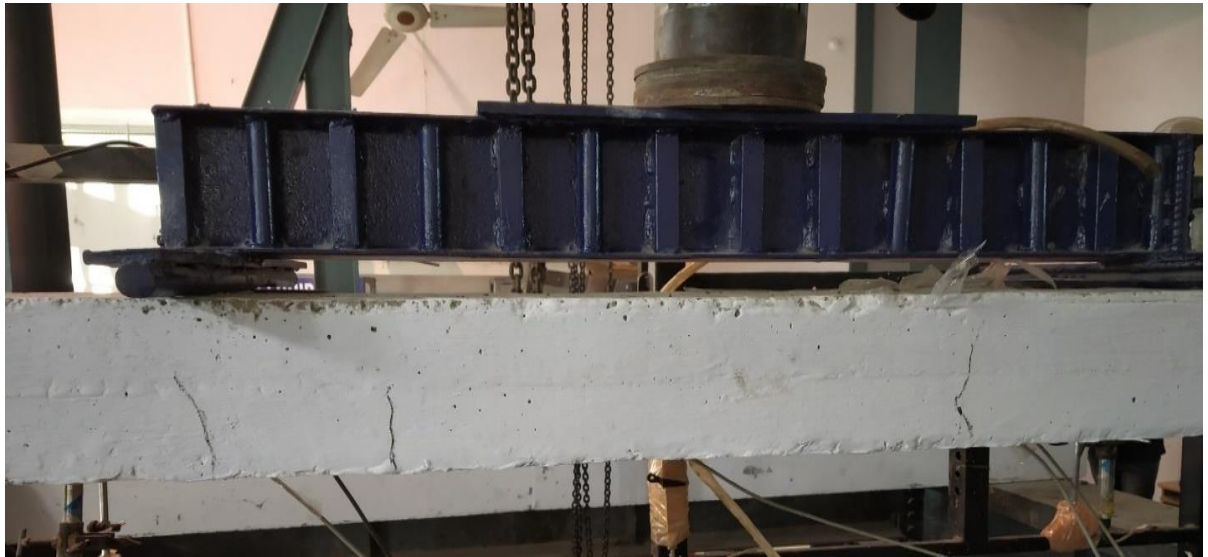
Fig.4.42 (a) Actual cracking at 2 nd cycle (SA)
