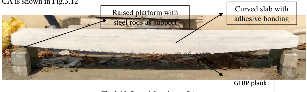
Fig.3.12 Casted Specimen CA
