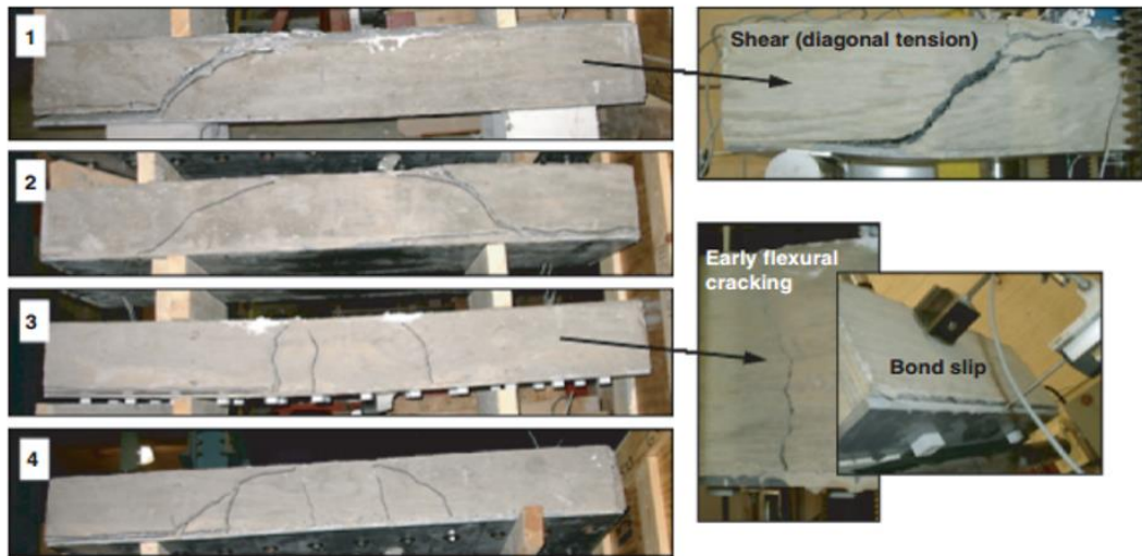
Fig.2.21 Failure Modes Specimens 1 to 4 ( Honickman et al. (2009) )
