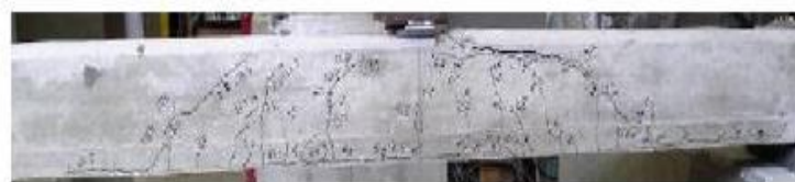
1) Hybrid failure mode of specimen 4
