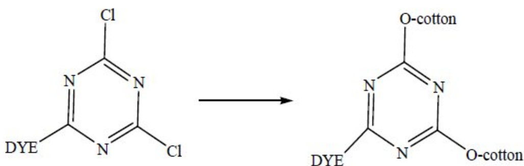
Fig. 2.1 Principle of cotton dyeing with a triazyl reactive dye (Kaur Sumandeep PhD. Thesis,(2008))
