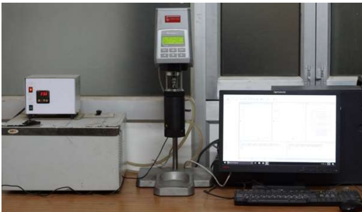
Figure 5.2: Rheolab Q-C (Rheometer) apparatus
