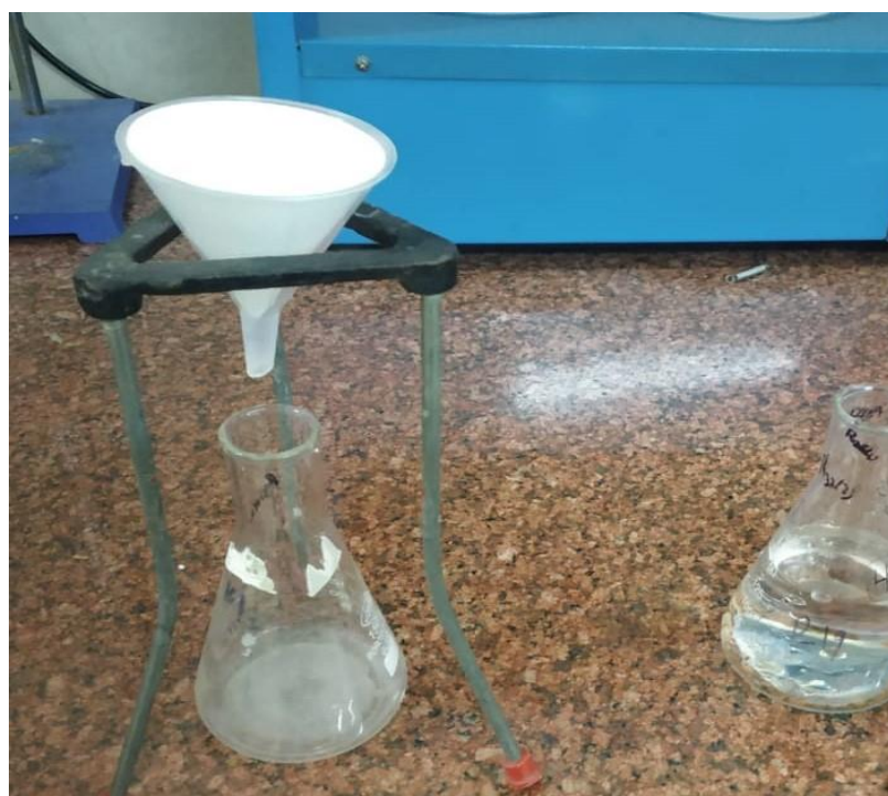
Fig. 4.11 Sulphate calculation by Gravimetric method (b)
