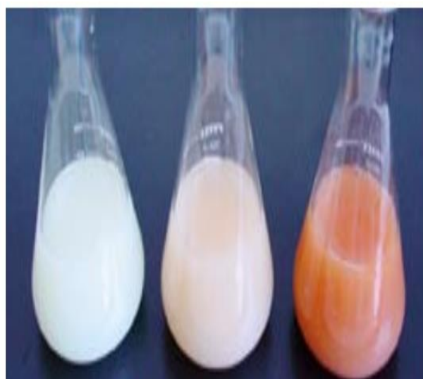
Fig. 4.6 Left flask shows before titration endpoint, it shows cloudy solution after adding \text{Ag}^+ ions; middle flask that all the \text{Cl}^- ions have precipitated; Right flask shows upon addition of \text{Ag}^+ ions after endpoint results in red-brown color solution.
