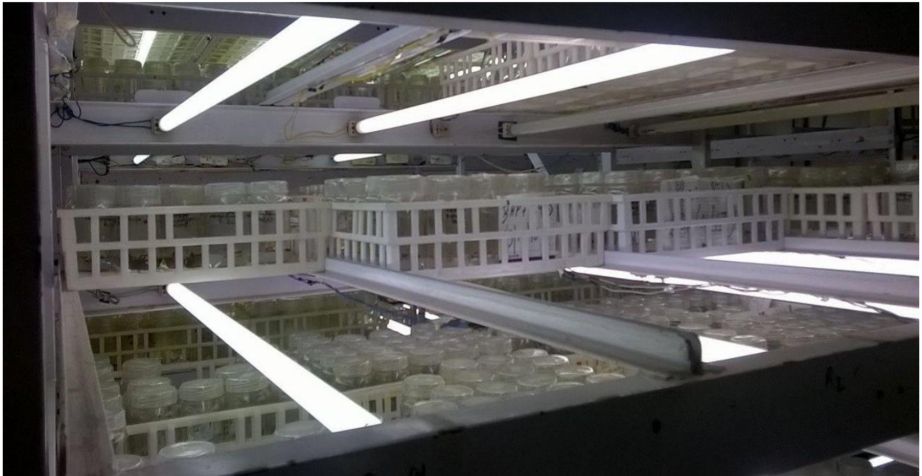
Fig.1.9. Use of fluorescent tube in tissue culture (Tiffacore, TIET).
