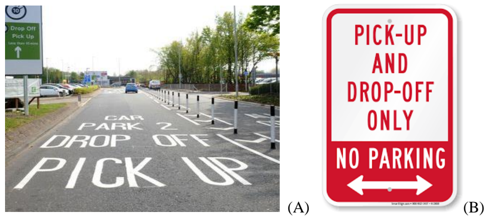
Figure 7.6 : (A) Pick up and Drop off Zone Pavement Marking (B) Pick up and Drop off Zone Sign
