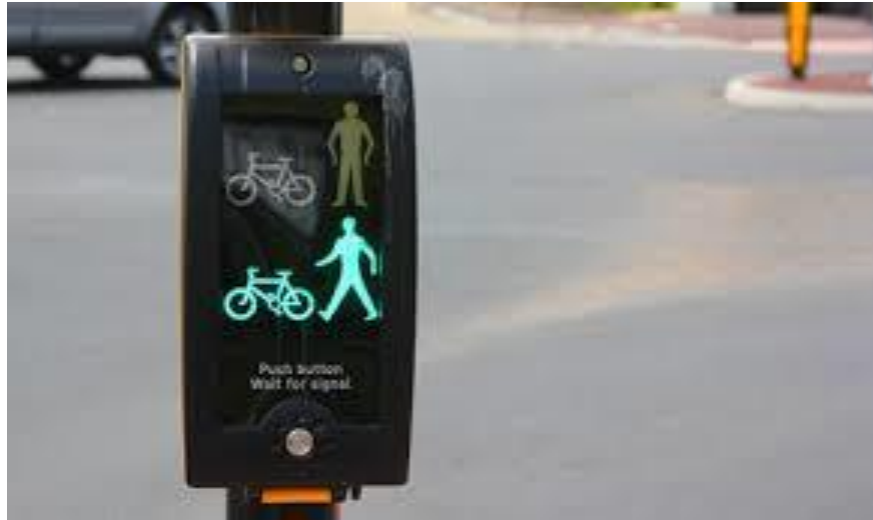
Figure 7.11 : Toucan Crossing for pedestrians as well as cyclist
