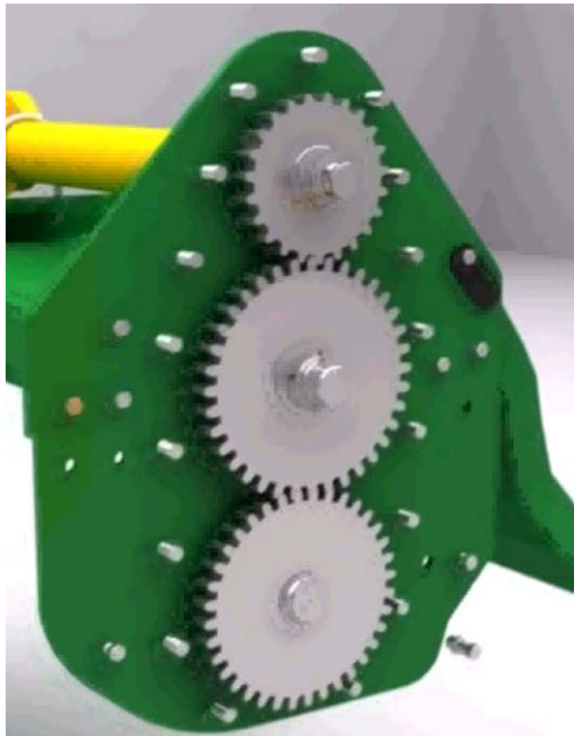
Fig. 1.2 Transmission system of the rotavator [23]
