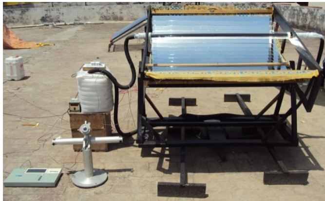
Figure 7.2 Parabolic trough collector with storage tank
