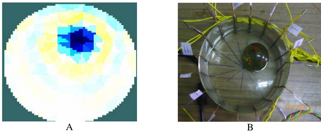
Figure 5.3: A Reconstructed Image of the Test Phantom. B Real photo of the test phantom.
