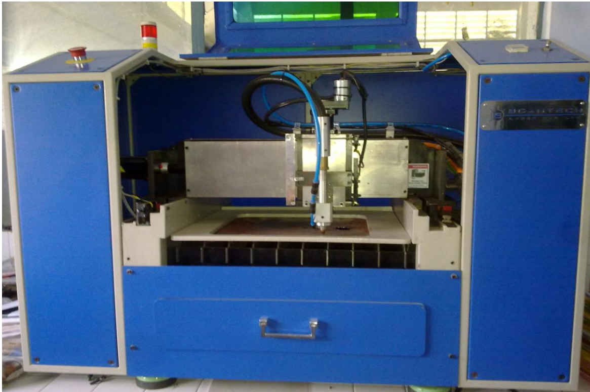
Fig. 3.2 Fiber Laser Beam Machine [Advanced machining lab, Thapar University]
