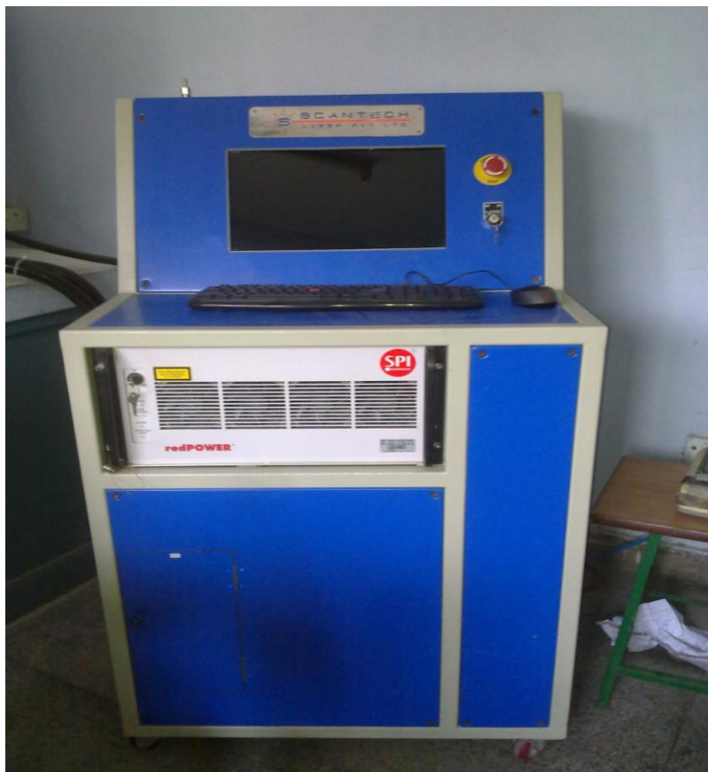
Fig. 3.3 Control Unit of LBM [Advanced machining lab, Thapar University]
