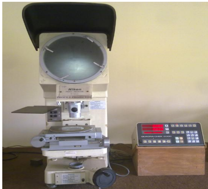
Fig. 3.4 Profile Projector [Metrology lab, Thapar University]
