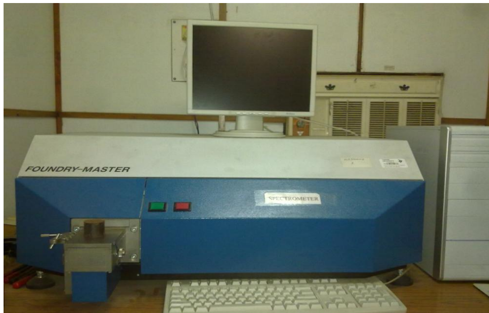
Fig. 3.5 optical emission spectrometer [Material testing lab, Thapar University]
