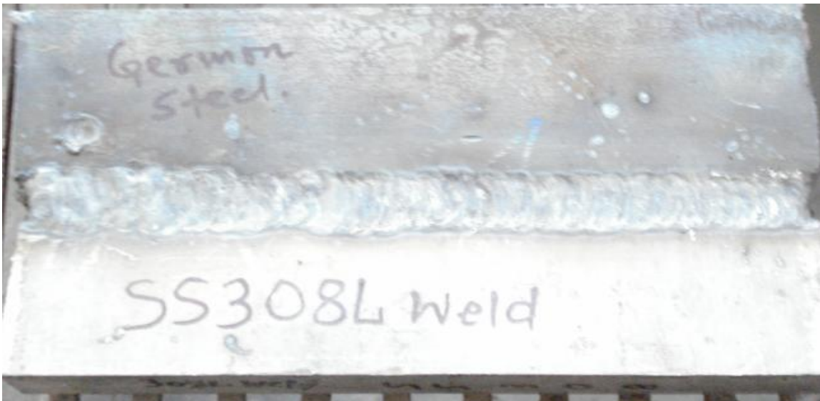
Fig 4.13 Welded plates of SS 308L without backing plate
