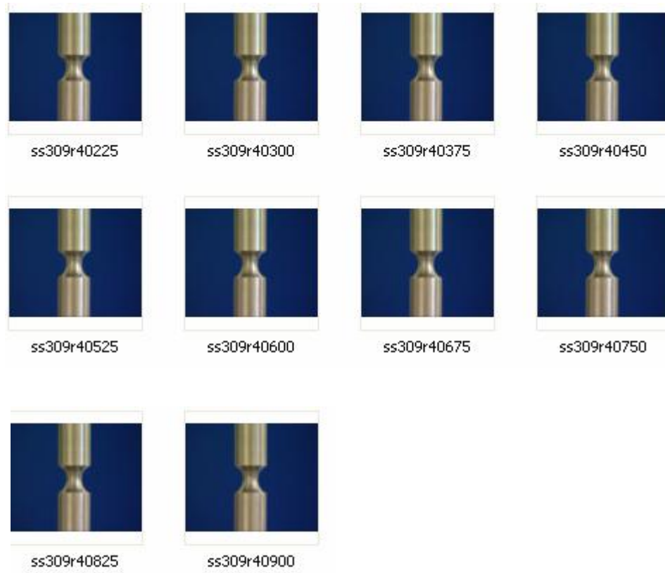
Fig 4.7 Photographs during testing of SS 309L R4
