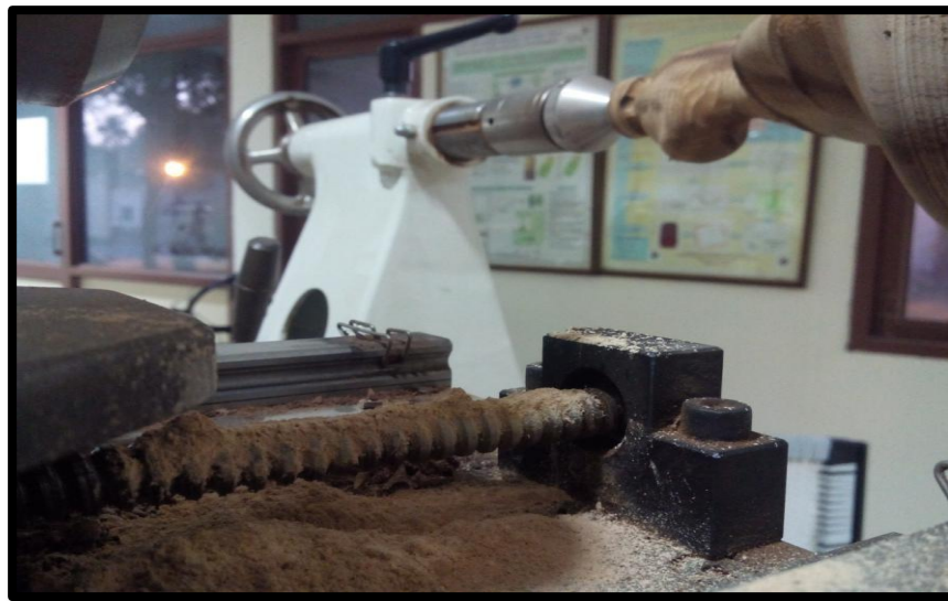
Figure 1.15: wood dust on ball screw
