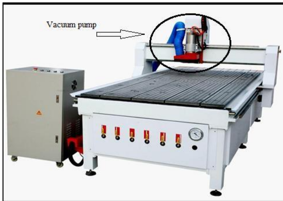
Figure1.16: A dust collection vacuum pump installed in machine [34]
