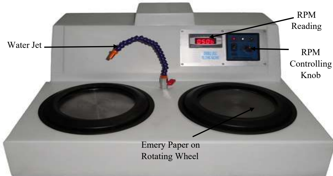
Figure 3.3 Disc polisher (Courtesy: CNC Lab, Thapar University)
