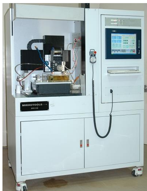
Figure 3.4: Micro tools DT 110, Singapore. Model: Multipurpose Micro machine
