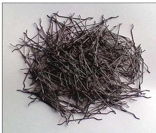
Plate 3.2: Hooked steel fibers used in the study
