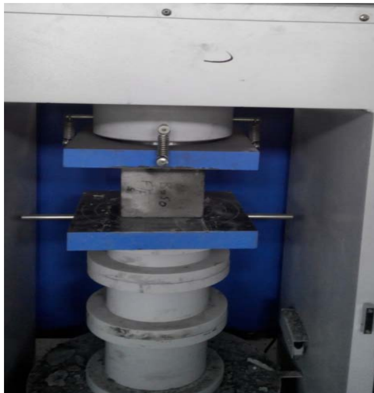
Plate 3.3: Compression testing machine used for study.
