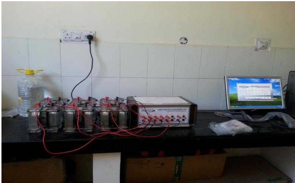
Plate 3.7: Rapid chloride permeability test set up (ASTM C 1202).
