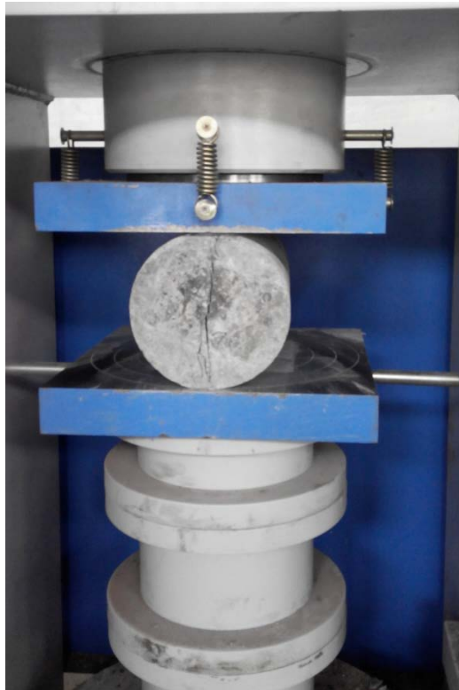
Plate 3.4: Splitting tensile strength testing machine used in the study
