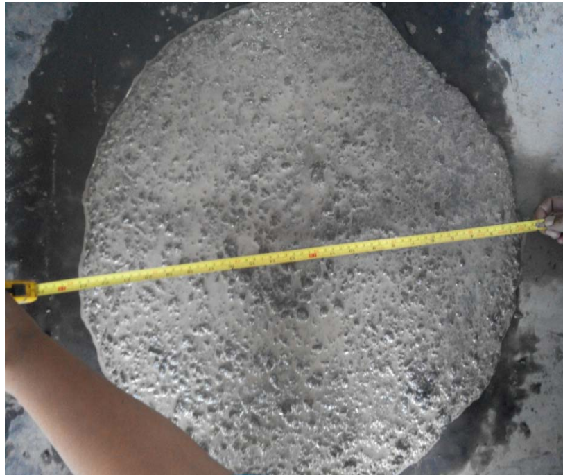
Plate 4.1: Achieved slum flow by slump flow test
