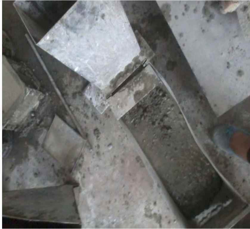
Plate 4.2: L- box test for fresh concrete
