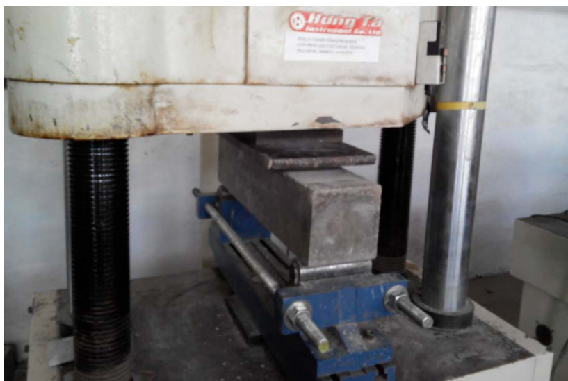
Plate 3.5: Flexural strength testing machine used in the study
