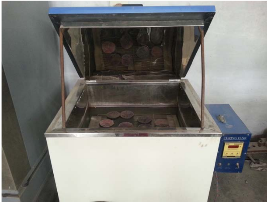
Plate 3.8: Samples boiled in curing tank at maintained temperature
