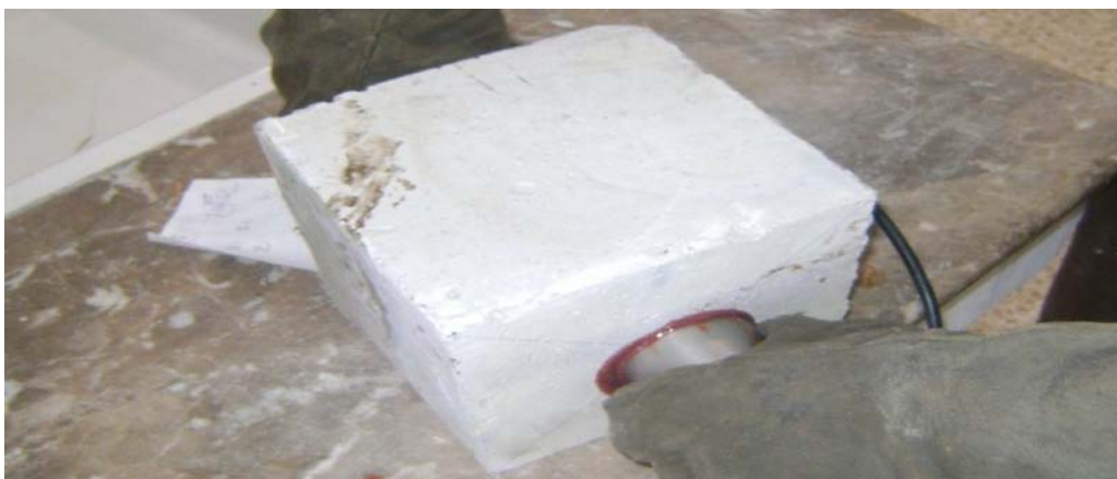
Plate 3.9: Pulse Velocity Test
