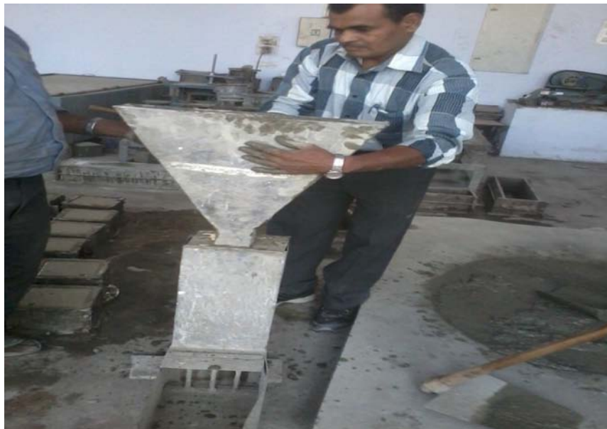
Plate 4.3: V-funnel test for fresh concrete
