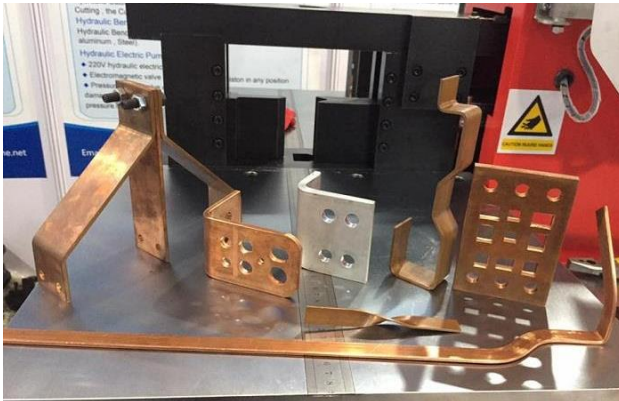
Figure 15, 16 Busbar shearing Bending and Punching Operation
