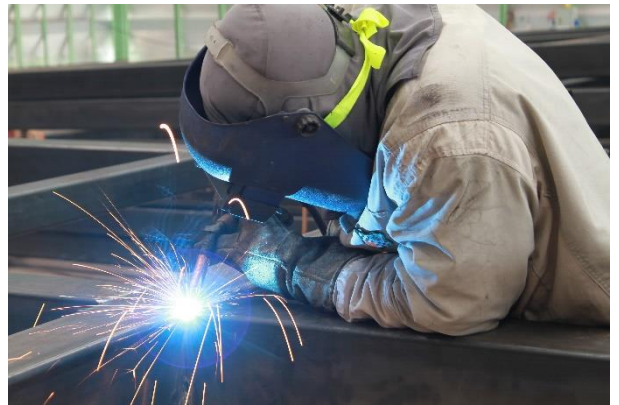
Figure 14 welding process by MIG welder
