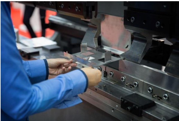
Figure 13 sheet bending at power press
