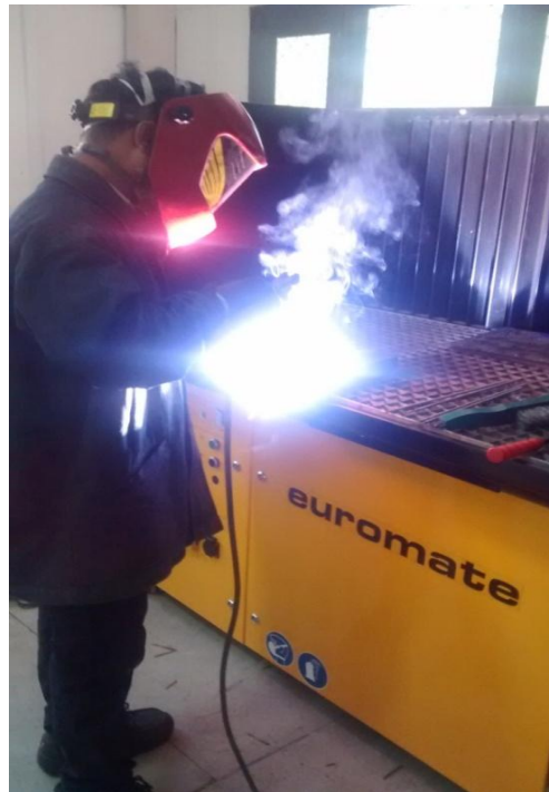
Figure 4.6.8 SMAW welding setup used.
