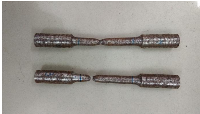
Figure A.7 Tensile specimens of MS buttering electrode.
