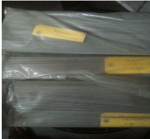
Figure 4.6.2 Core wires used for the development of coated electrodes.
