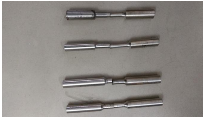
Figure A.8 Tensile specimens of SS304L.
