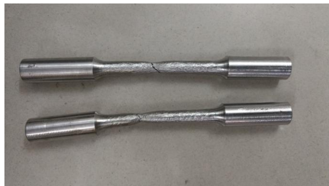
Figure A.9 Tensile specimens of welds (three layer methodology).
