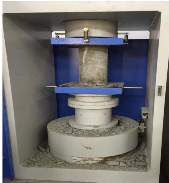
Fig. 4.3: Test set-up for measuring compressive strength of RCC
