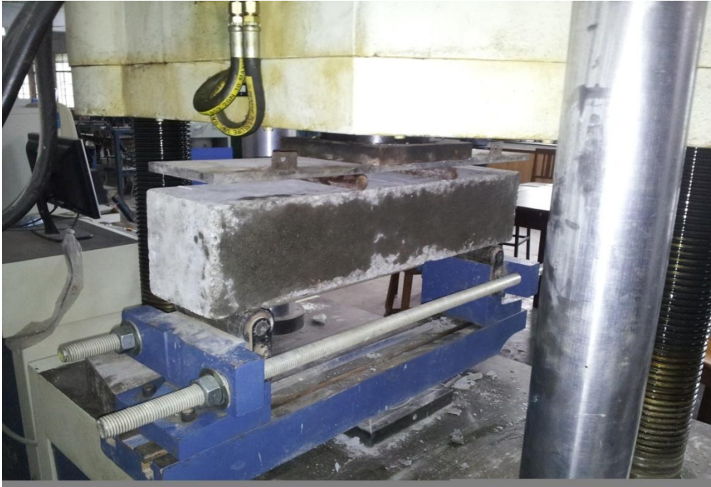
Fig. 4.5: Test setup for measurement of flexural strength of the RCC
