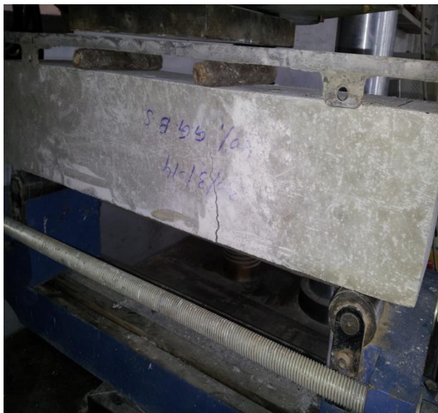
Fig. 4.6: Beam specimens after fracture showing the crack position
