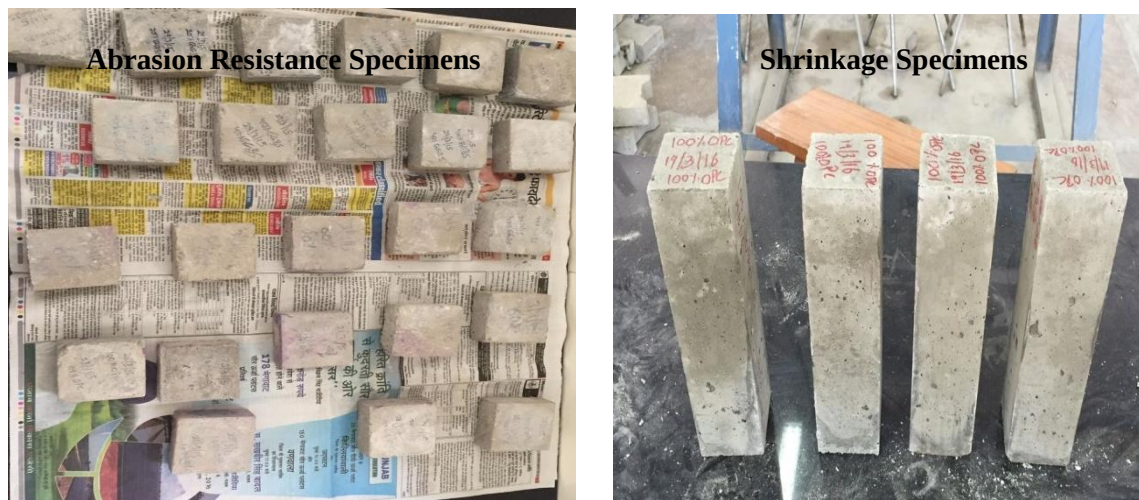
Fig. 5.2: RCC blocks for abrasion resistance measurement and prisms for shrinkage properties
