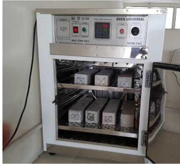
Fig. 5.5: Temperature control chamber with prism specimens
