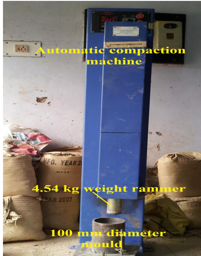
Fig. 3.10: Compaction arrangement for determination of moisture –density content
