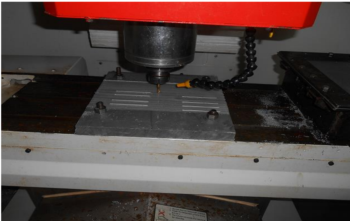
Figure 4.2: Experimental setup of machined workpiece showing various values of axial and radial depth of cuts.
