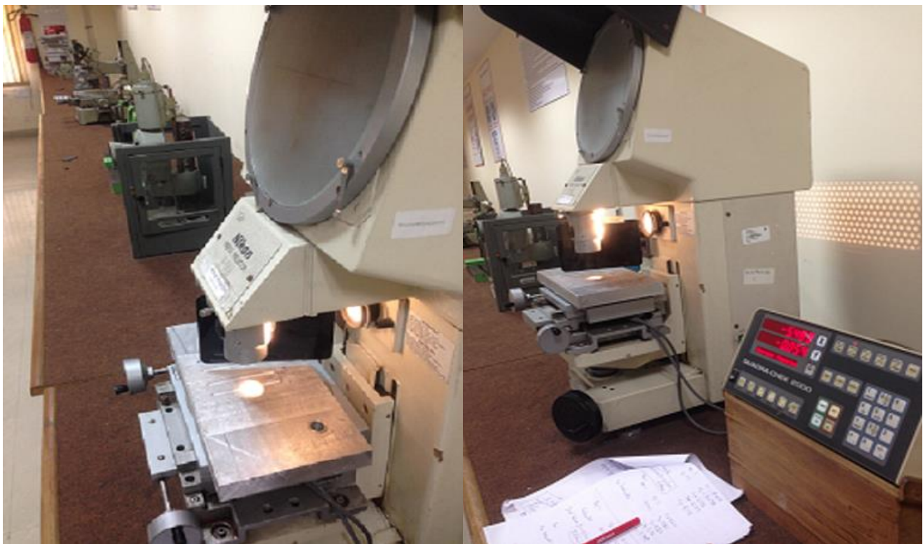
Figure 4.4 Measurement of compensated and non-compensated slots on profile projector
