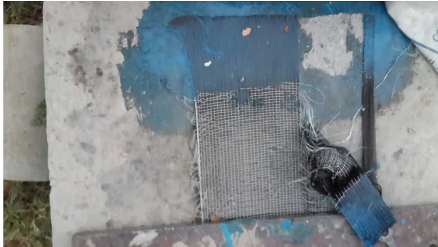
Fig.4.6 Sample S11 Failed due to Concrete Shear
