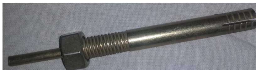
Fig 3.8 12 mm Anchored Bolts Used for Fastening Prestressed Machine
