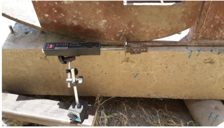
Fig 3.12 LVDT Placed to Measure The Elongation in FRP Sheet
