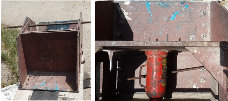
Fig 3.5 Prestressing Machine in Right and Hydraulic Jack in Left to Move the Rotating Arm
