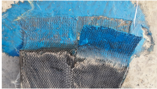
Fig.4.3 Failure of Sample S6
