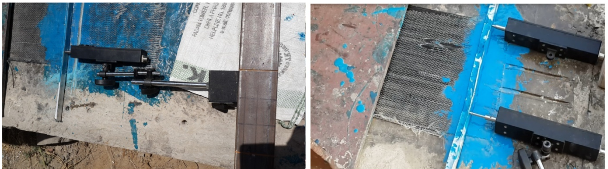
Fig 3.11 LVDT's for the Measurement of Slips in FRP With Reference To Aluminium Angle
