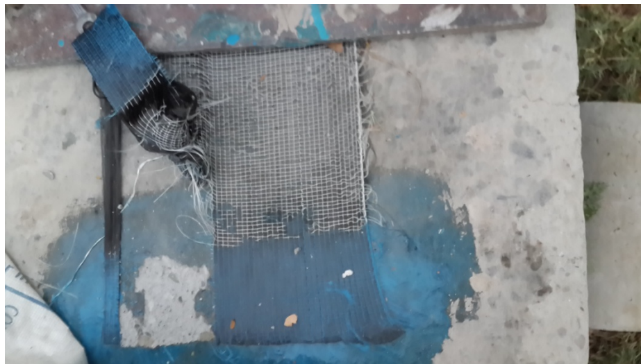
Fig. 4.5 Failure of Sample on Undamaged Beam S10
