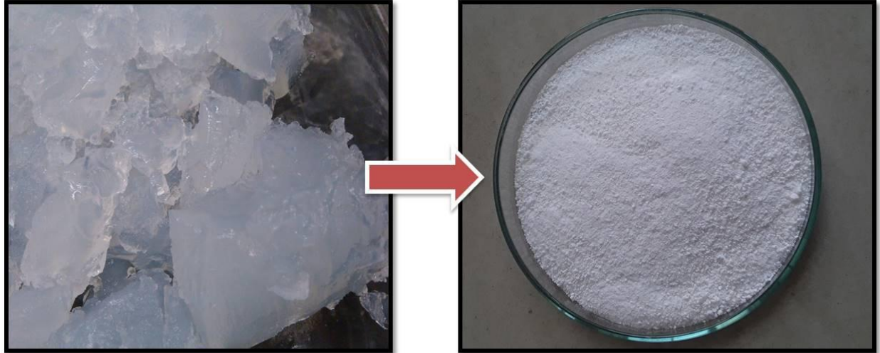
Figure 4.5: Obtained silica after jelly dried at 100°C.
