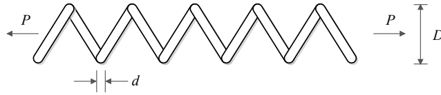
Fig. 3.9. Schematic view of tension/compression spring problem.
