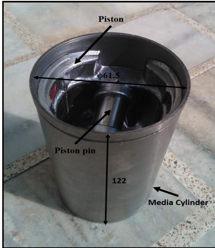
Figure 3.5: Media cylinder & piston arrangement
