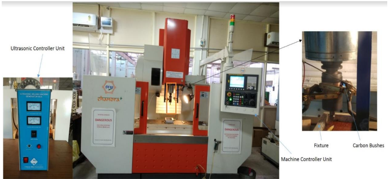
Figure A-3: 3-axis vertical milling center (Courtesy: CNC lab, Thapar Institute of Engineering & Technology, Patiala)
