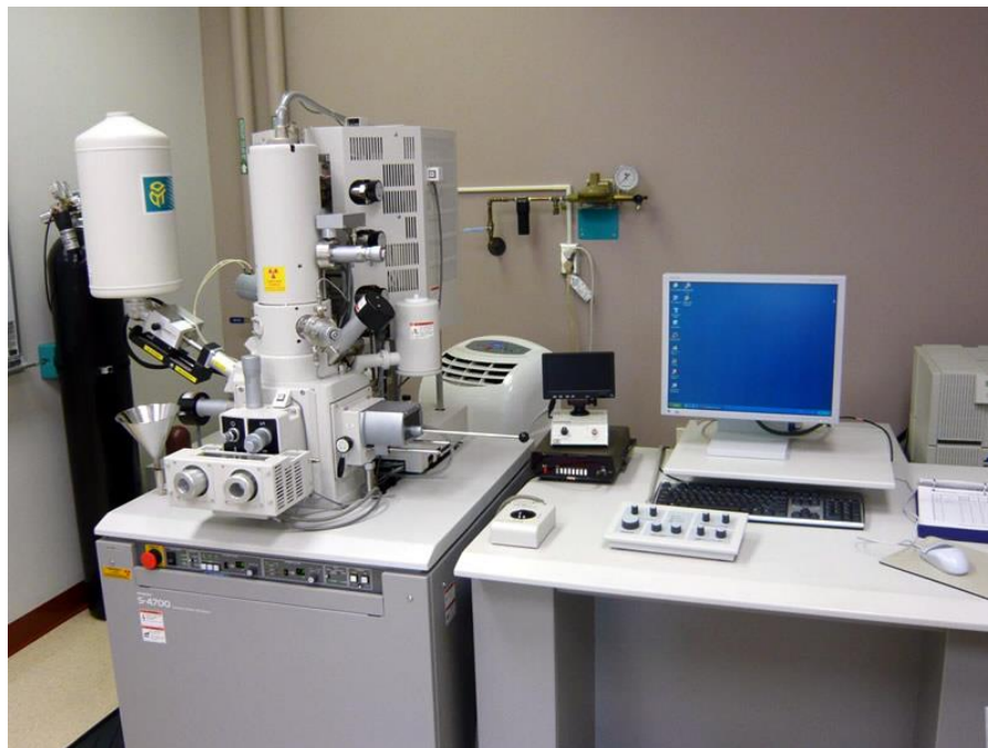
Figure A-2: Scanning Electron Microscopy (SEM) (Courtesy: SAI lab, Thapar Institute of Engineering & Technology, Patiala)
