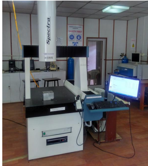
Figure A-1: Coordinate Measuring Machine (Courtesy: Advanced metrology lab, Thapar Institute of Engineering & Technology, Patiala)
