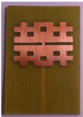
Figure 6.3 Front view of Antenna
