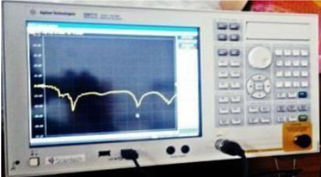
Figure 6.6 Network Analyser with antenna connectivity for Testing
