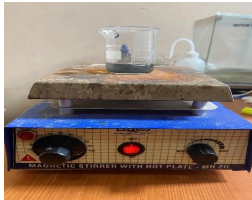
Figure 3.2: Illustration of magnetic stirrer equipment
