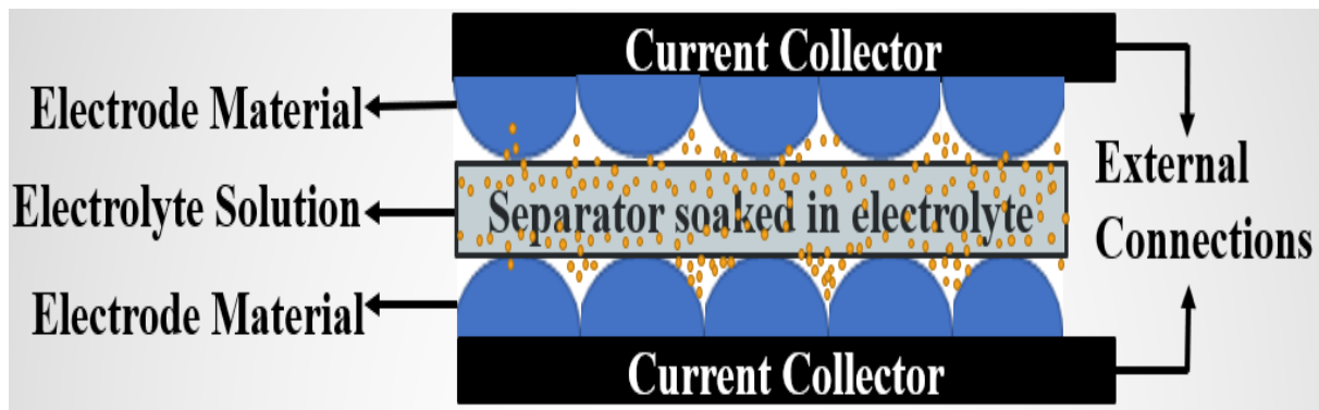
Figure 1.3: Schematic diagram of supercapacitor
