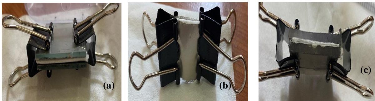
Figure 4.3: Fabrication of symmetrical supercapacitor device on (a) Glass, (b) PP, and (c) PET substrates.
