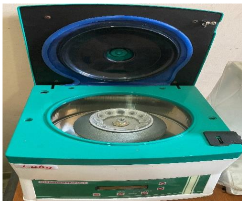
Figure 3.15: Diagram illustrating the centrifuge equipment.
