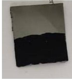
Figure 5.2: Fabrication of electrode material on graphite sheet.
