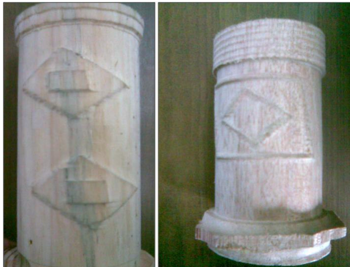
Figure 4.14: (a) Extruded portion on the cylindrical base (b) Sweep pattern
