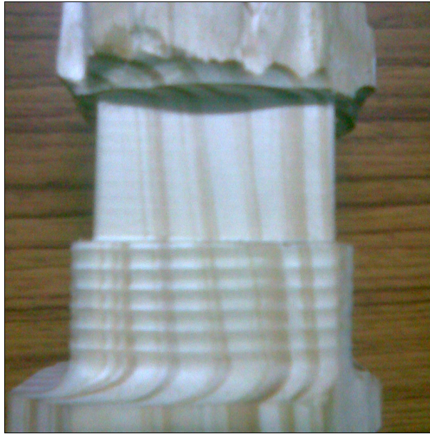
Figure 4.11: Square prism with roughing and finishing passes shown
