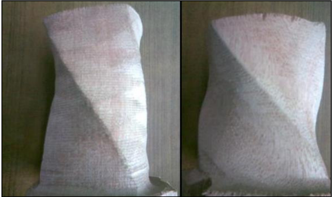
Figure 4.13: (a) Twisted prism with rough pass and (b) Twisted prism with finished pass
