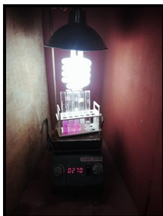
Fig24 Degradation of RhB using the nano-composite ( SnO 2 /C 3 N 4 )
