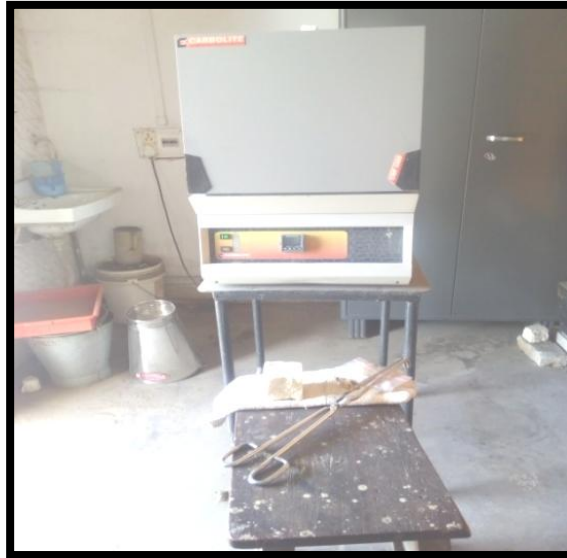
Figure 3.15: Carbolite furnace used for baking of pre-strained processed specimens (Courtesy: NML Jamshedpur).
