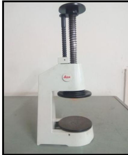
Figure 3.11: Leveling Machine (Courtesy: NML, Jamshedpur).
