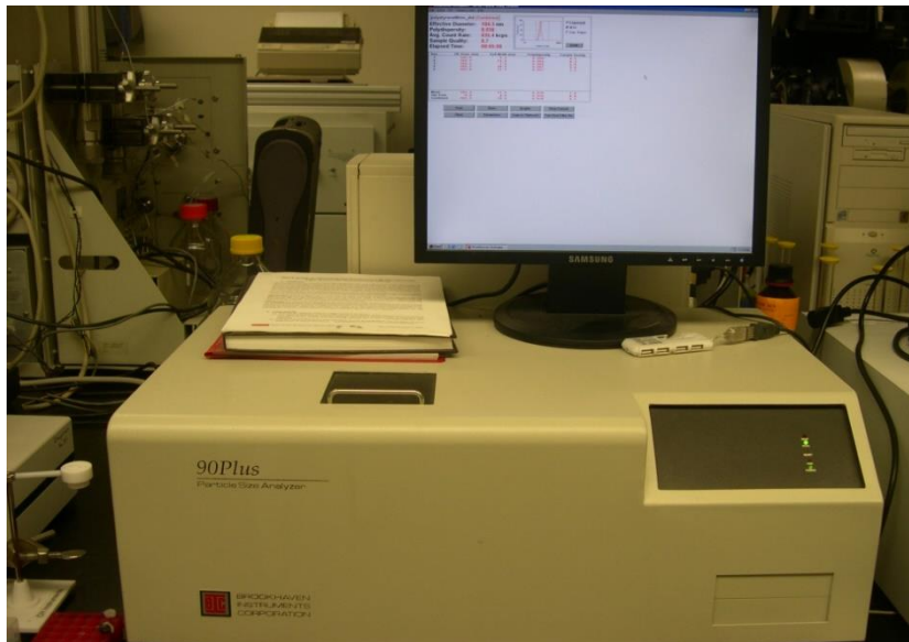
Figure 3.5. Photographic view of Dynamic light scattering setup (90 Plus particle size analyzer from Brookhaven Instruments).
