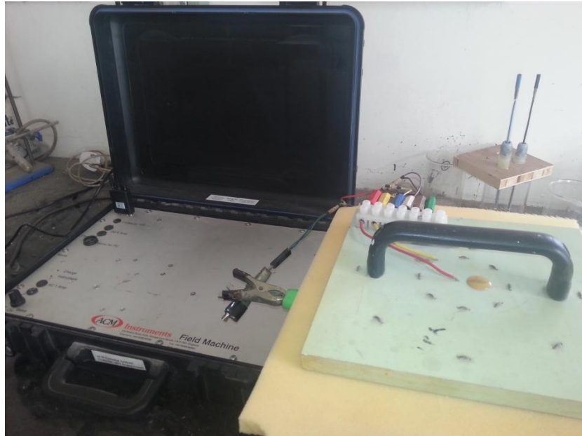
Fig.4.8: Guard ring arrangement for measuring I_{corr}
