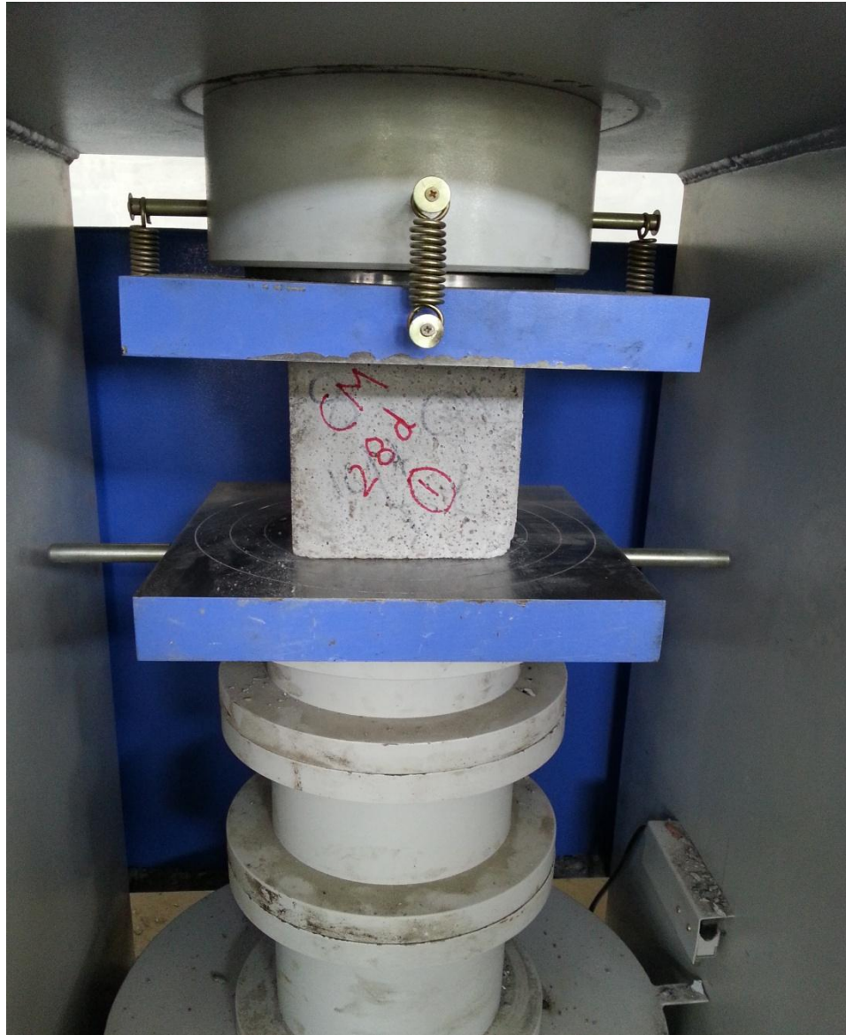
Fig.4.7: Testing for compressive strength
