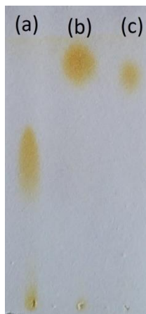
Fig.1. TLC analysis of (a) waste cooking oil ( R_f = 0.4 ), (b) waste cooking oil derived FAME ( R_f = 0.7 ) and (c) methyl oleate standard ( R_f = 0.7 ).
