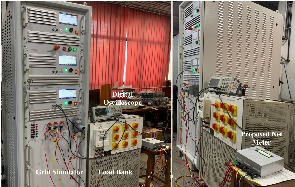
Figure 3.9: Test bench 1 configured for VT, CT and FFT testing is shown with the front and side view.
