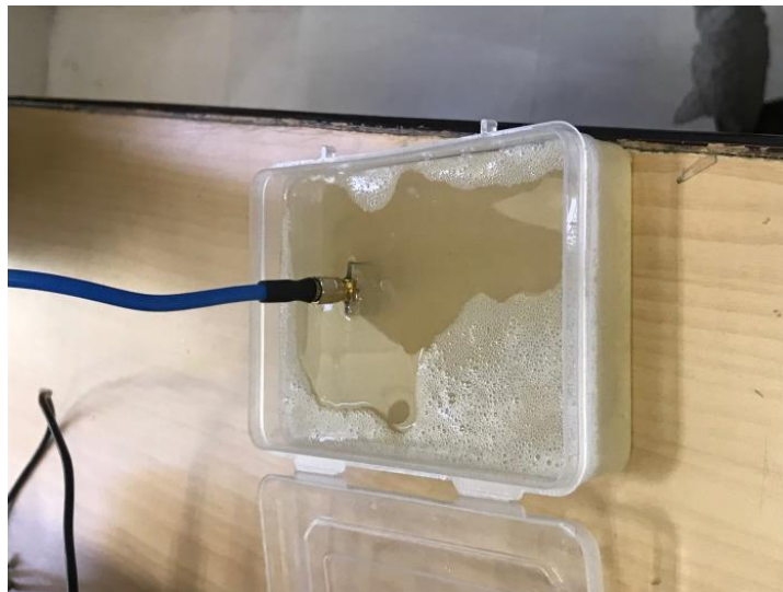
Figure 6.4 Fabricated Antenna embedded in Skin mimicking material
