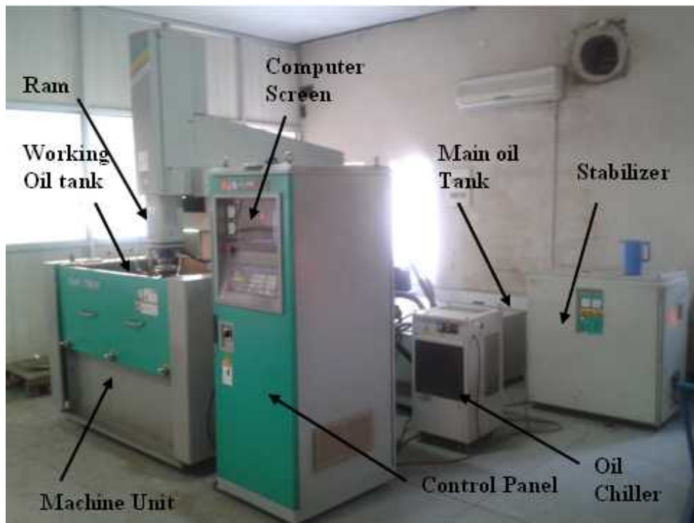
Figure 3.1: Pictorial View of EDM Machine used for the Experimentation
