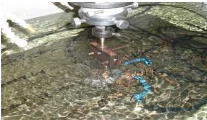
Figure 3.2: (a) Alignment of Electrode, (b) Tool and Workpiece set-up, (c) Tool and Workpiece Sink in Dielectric Liquid and (d) Actual Operation Performed in Dielectric
