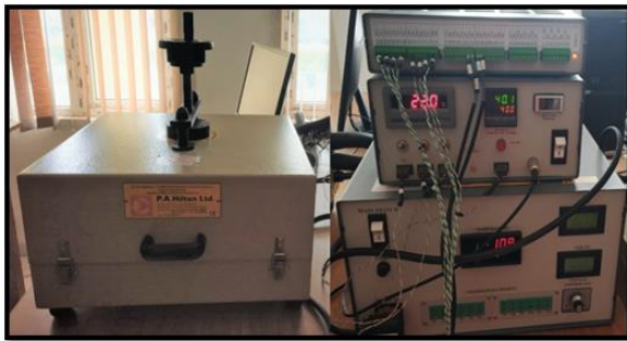
Fig. 1 Shows the thermal conductivity measurement setup with PID controller.
