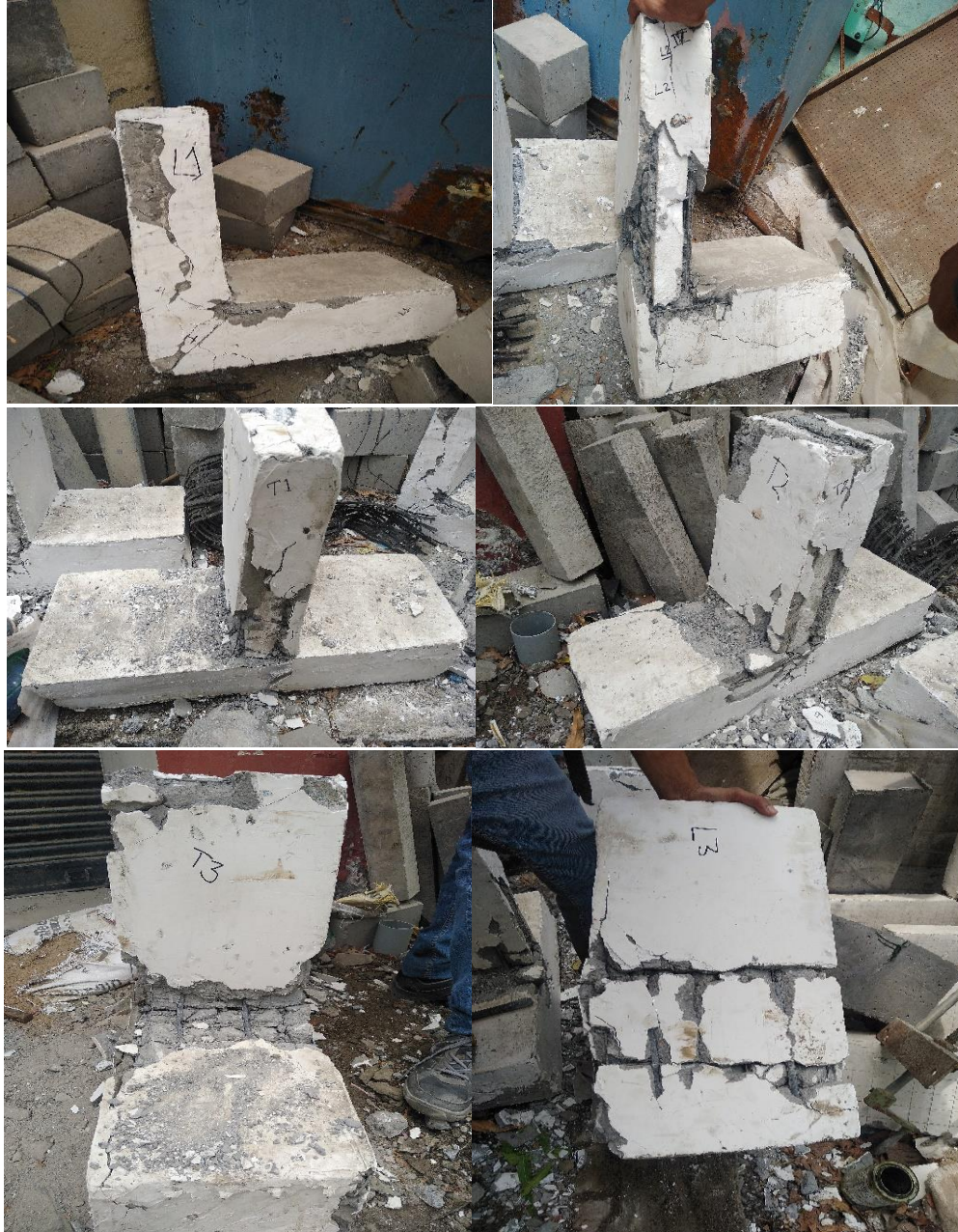
Figure B1 Crack pattern in different specimens after testing
