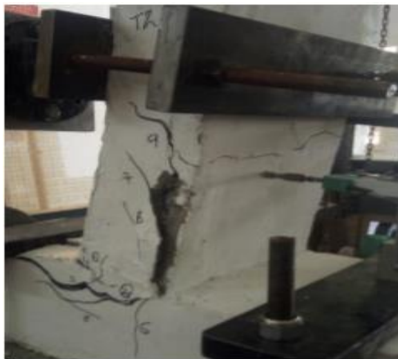
Figure 4.8 Crack pattern in T2 during testing
