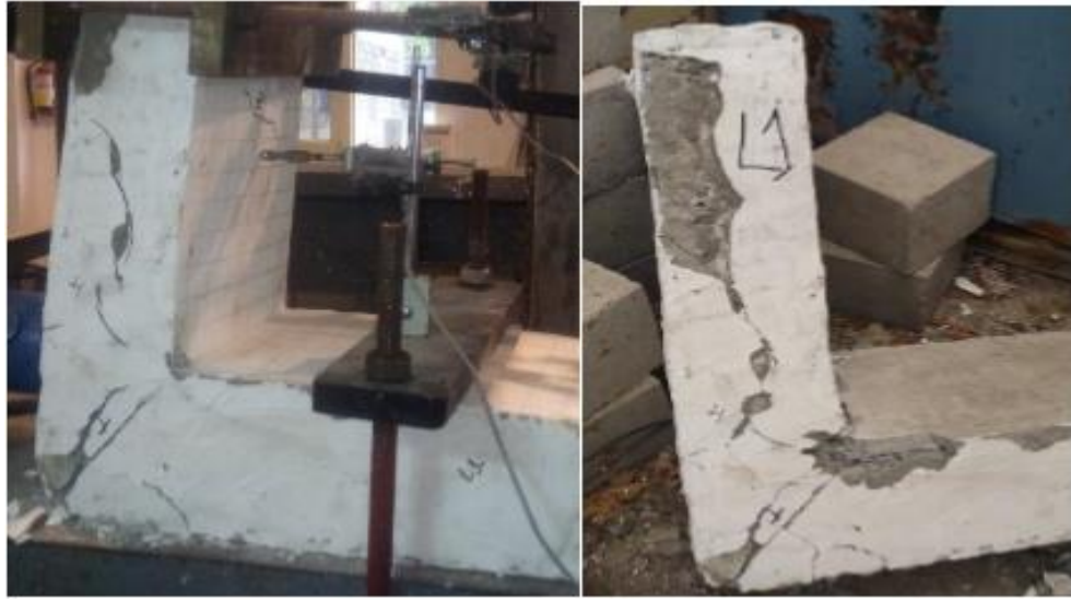
Figure 4.2 Cracks developed in L1 during testing
