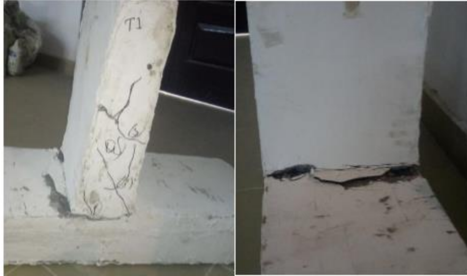
Figure 4.7 Crack pattern in T1 during testing
