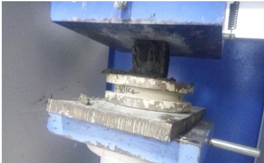
Figure 3.6 Compression testing of a cement mortar cube
