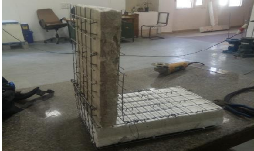
Figure 3.13 Wall and Slab 3D panels tied up using L-shaped mesh
