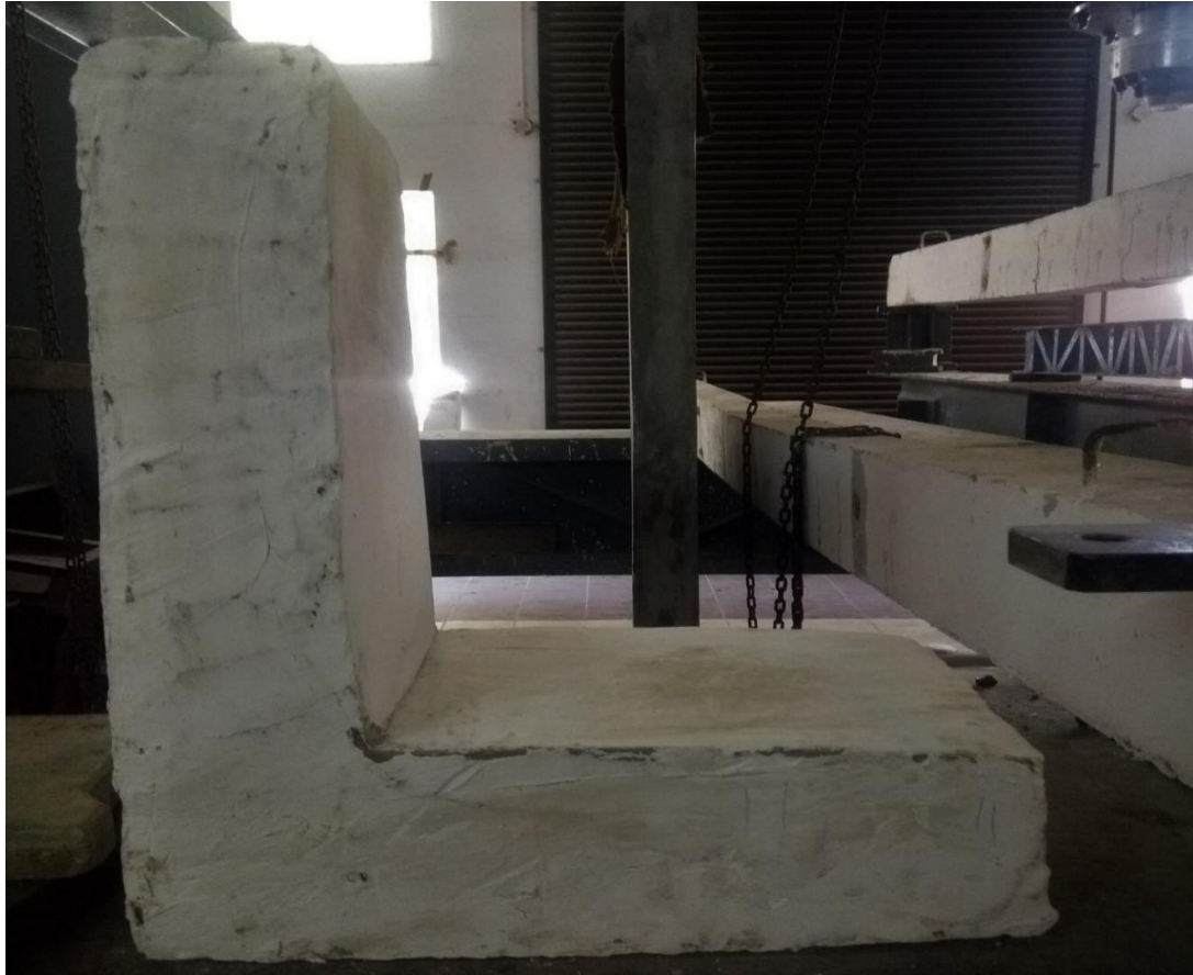
Figure 3.15 Fully finished L-shaped connection after 28 days of casting
