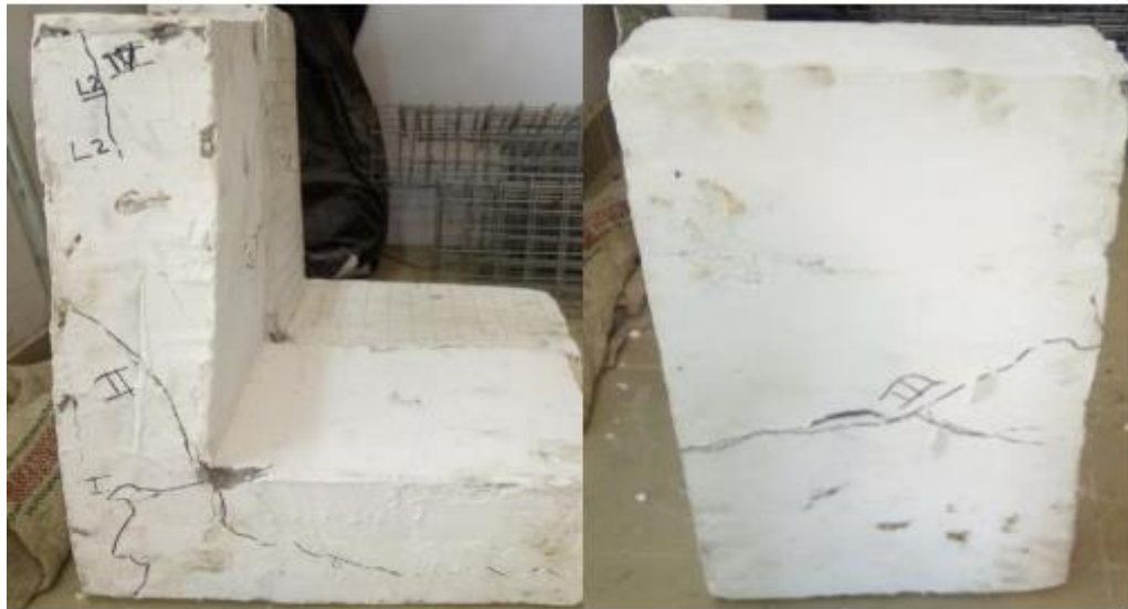
Figure 4.3 Cracks developed in L2 during testing
