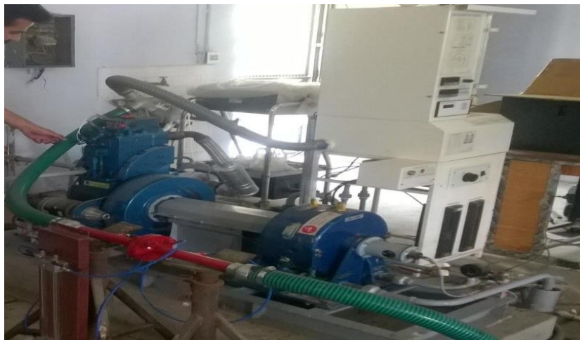
Fig 3.10: Dual fuel engine setup coupled with a dynamometer
