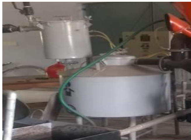
Fig 3.7: Filters for ultra-cleaning of the gas
