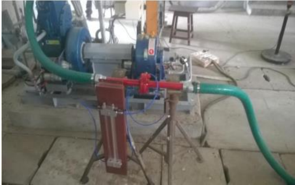
Fig 3.9: Flow meter used to measure flow rate of producer gas.
