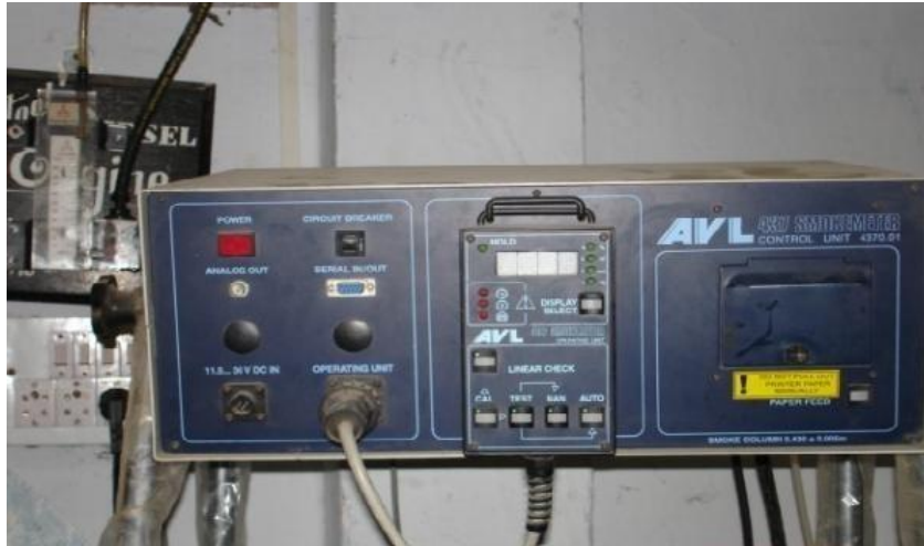
Fig.3.13: AVL smoke meter used for smoke opacity
