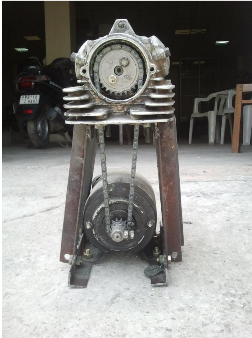
Fig 3.3 Set up for measuring cam chain noise
