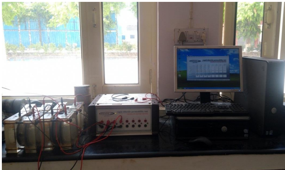
Figure 3.6 : Rapid Chloride-ion Permeability Test
