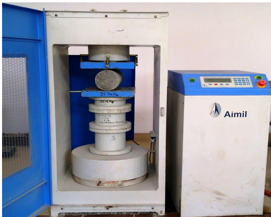
Fig. 3.4 : Splitting Tensile Strength Test of Concrete
