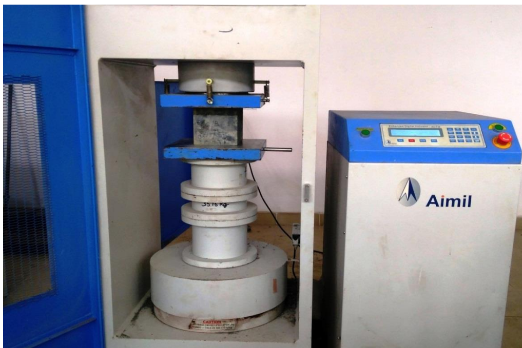
Figure 3.3 : Compressive Strength Test on Compression Testing Machine
