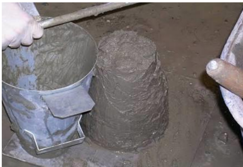
Figure 3.2 : Slump Test of Concrete
