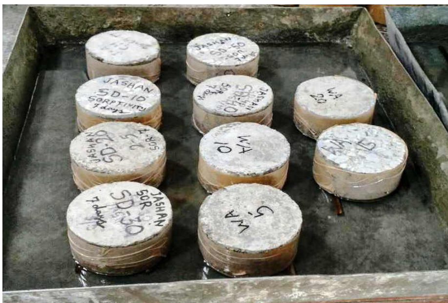
Figure 3.5 : Sorptivity Test of Concrete Samples
