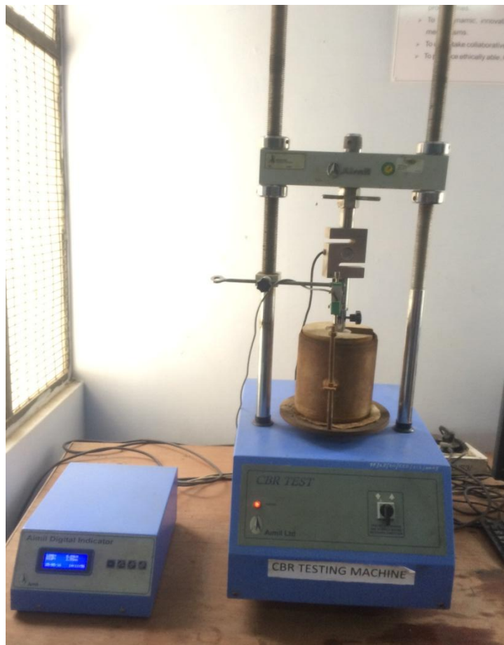
Figure 3.4: California bearing ratio testing Machine
