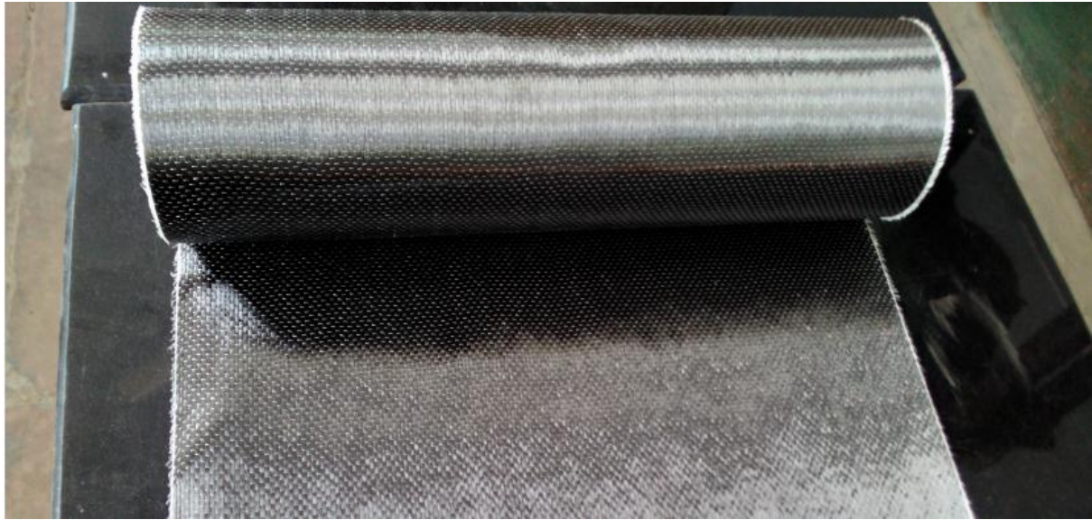
Figure 3.1 – CFRP sheet used for strengthening of beams
