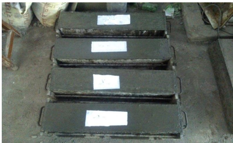
Figure 3.4 – Beam specimens at the time of casting
