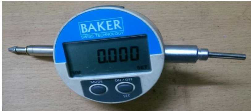
Figure 3.2 – Dial gauge used for measuring the deflection
