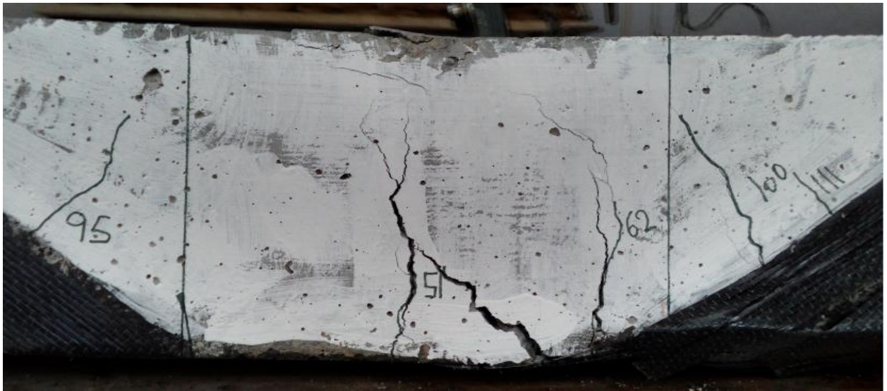
Figure 4.23 – Crack patterns in strengthened beam SB-09
