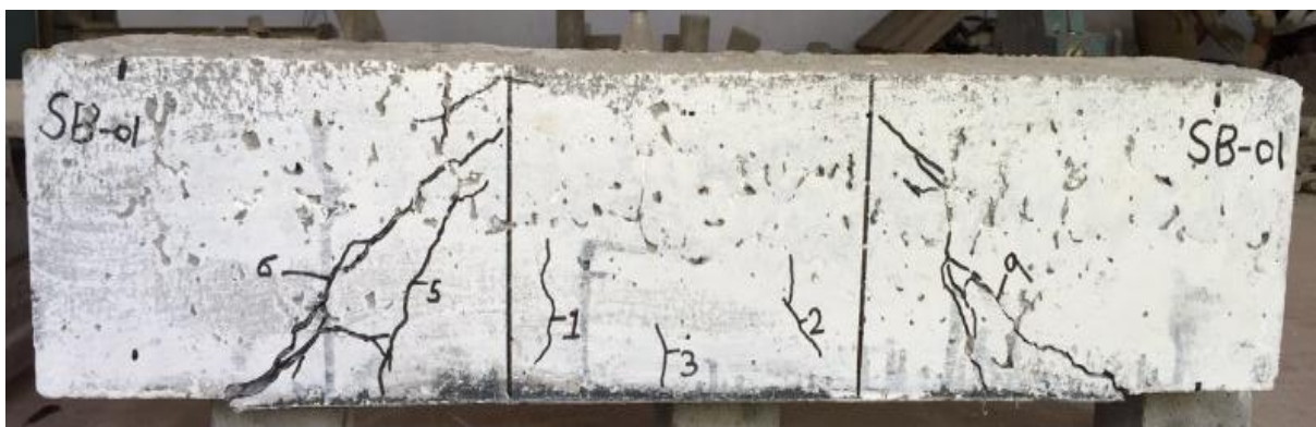
Figure 4.7 – Crack patterns in strengthened beam SB-01
