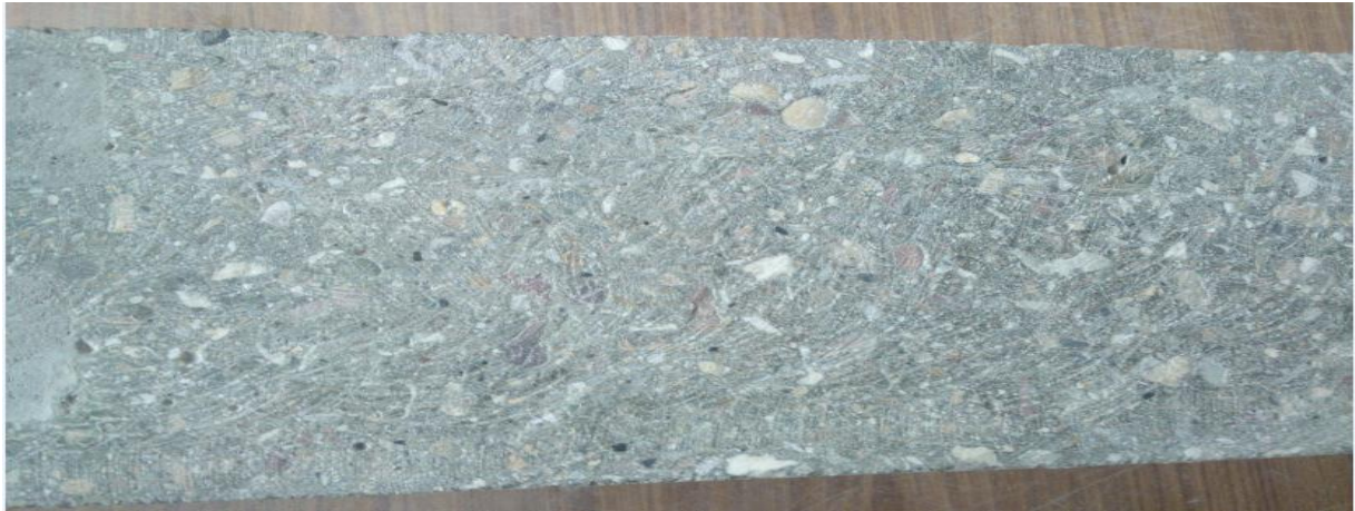
Figure 3.5 – Surface of beam after grinding
