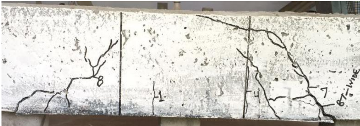
Figure 4.9 –Crack patterns in strengthened beam SB-02
