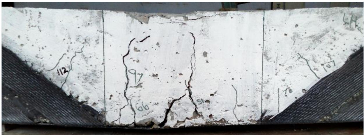
Figure 4.19 – Crack patterns in strengthened beam SB-07
