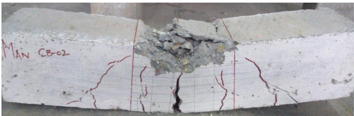
Figure 4.4 – Failure of control beam CB-02
