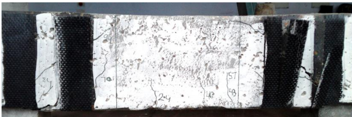
Figure 4.11 – Crack patterns in strengthened beam SB-03
