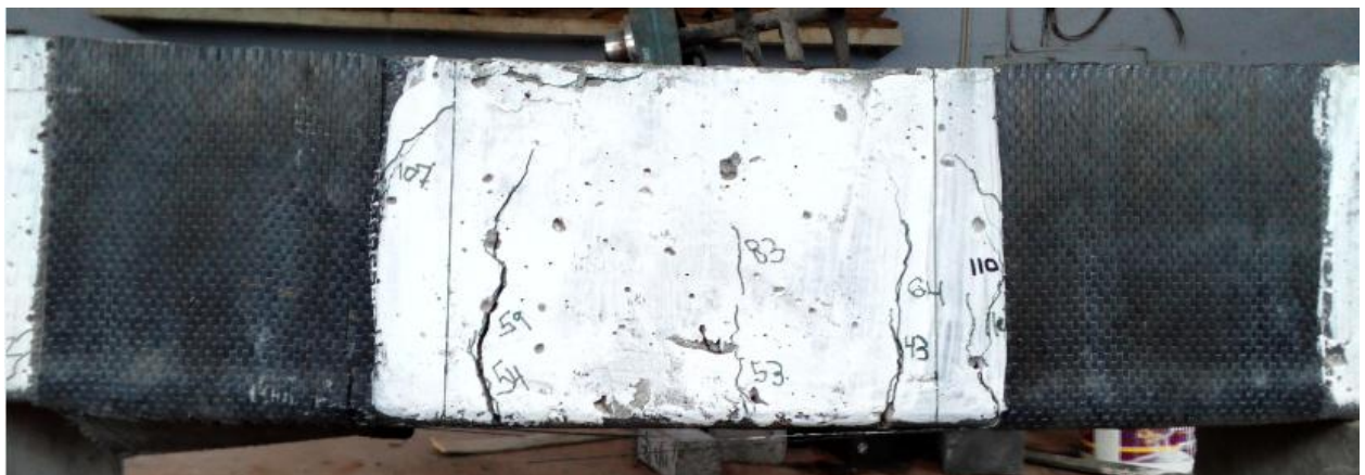
Figure 4.27 – Crack patterns in strengthened beam SB-11
