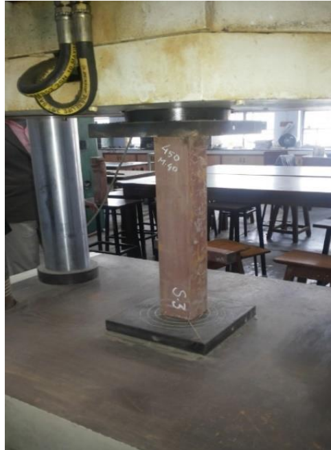
Figure 3.3. Test Set-Up for Axial Compression Testing
