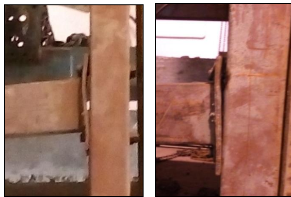
(c) End Plate Deformation of SR-EPTB and SR-EPAB
