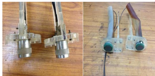
(c) Immersion probes (left) 0.5 MHz (right) 1 MHz
