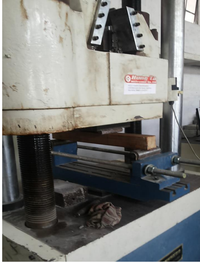
Figure 6.21 Flexural Testing Set-Up
