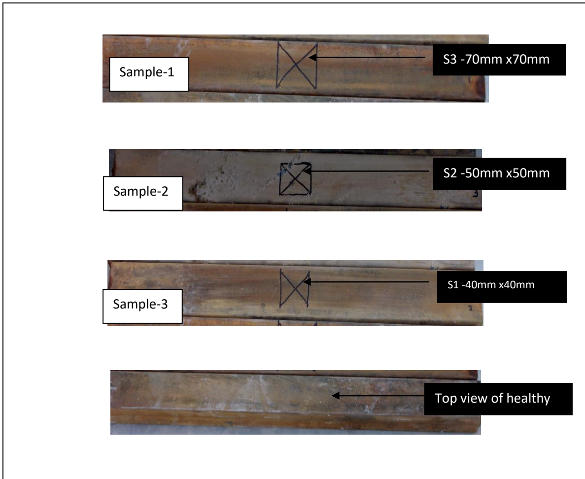
Figure 6.7 Simulated Debond Specimens
