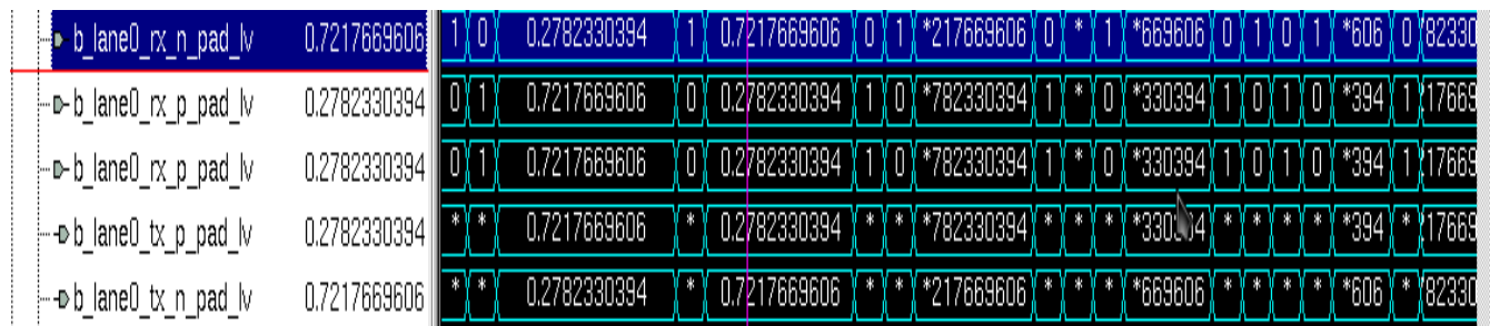
Figure 7.4 Output at pad with loopback performed
