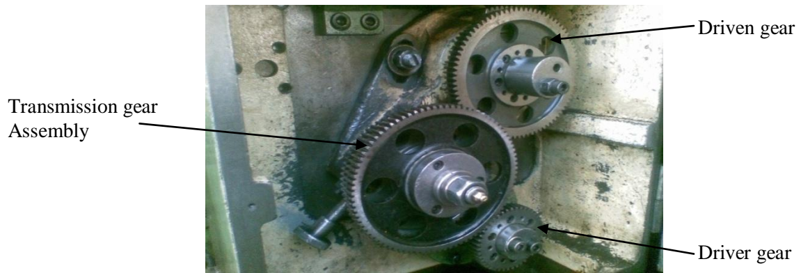
Figure 4.10: Feeder gear box assembly [Crompton Greaves, Ahmednagar]
