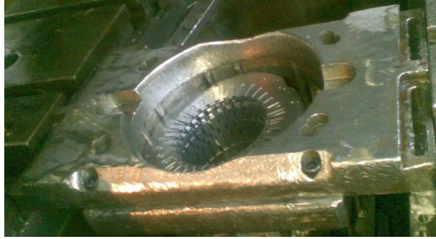
Figure 6.4: Existing stator chute plate [Crompton Greaves, Ahmednagar]
