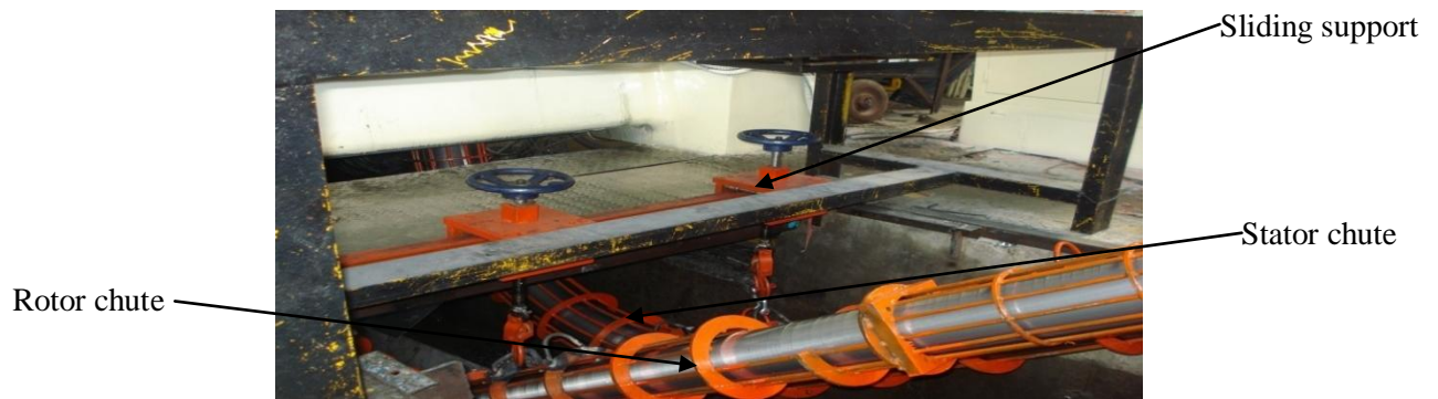
Figure 6.32: Final assembly of sliding support attached with chute [Crompton Greaves, Ahmednagar]
