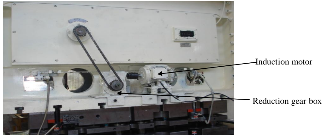
Figure 7.4: Motor and reduction gear box assembly attached with slide
