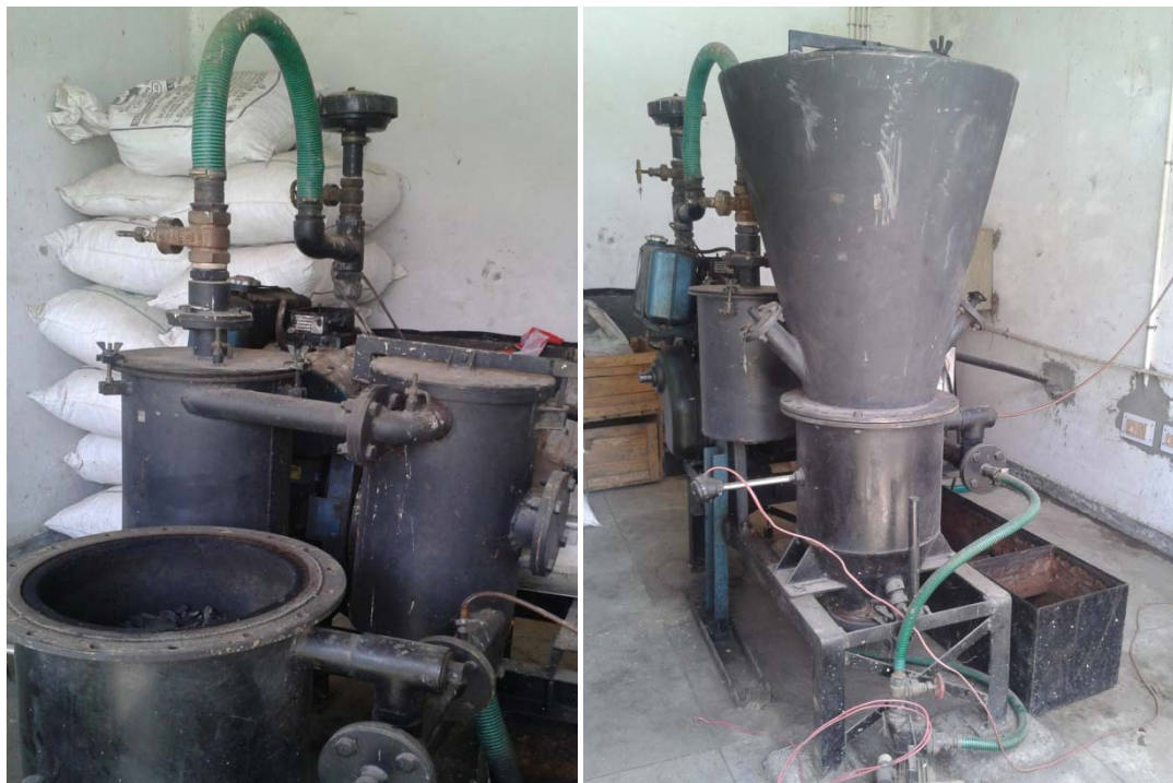
Fig. 4.2 Reactor filled with charcoal and gas cleaning filters and hopper reactor system coupled.
