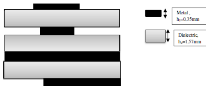
Figure 6.1: side view of the antenna showing its layered structure
