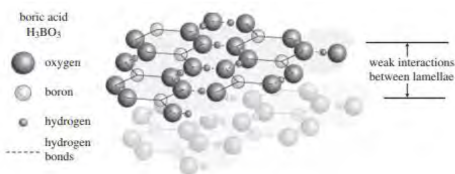
Figure 1.5: Lamellar structure of boric acid [44]
