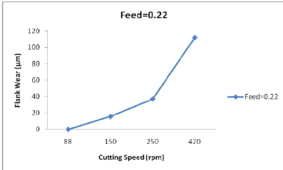
Fig. 5.8 Cutting Speed Vs Flank Wear at 0.22 Feed
