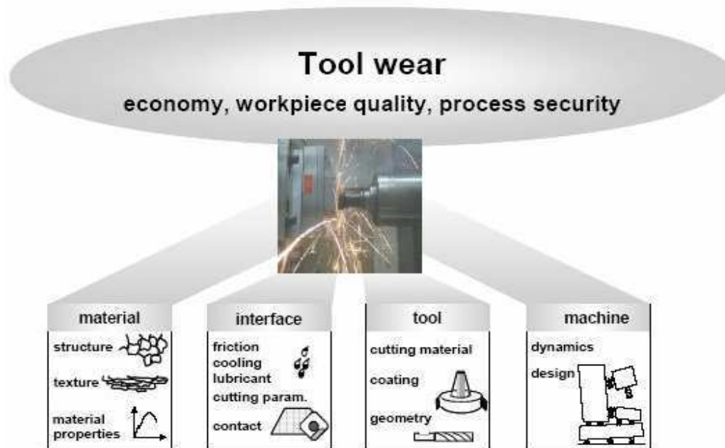
Fig. 3.3 Influencing elements of tool wear [24]
